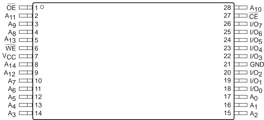
TSOP Top View (8mm X 13.4mm) (T13)
