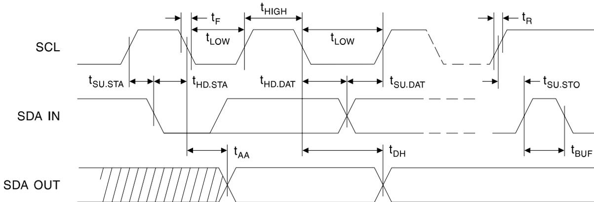
**Write Cycle Timing (SCL: Serial Clock, SDA: Serial Data I/O)**
