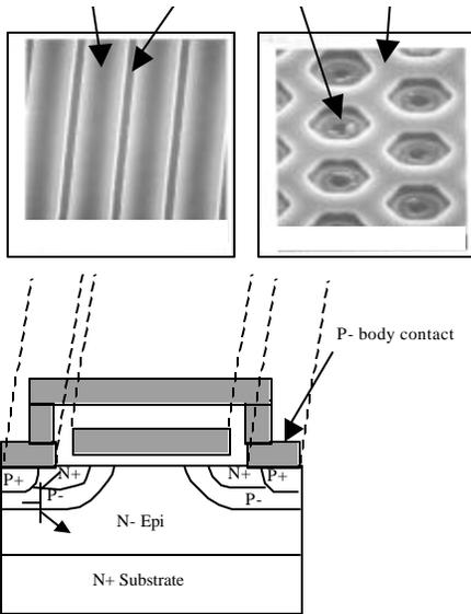
Fig. 9. Photo of the novel planar versus older cell topology and cross-section of power MOSFET showing parasitic bipolar transistor.
