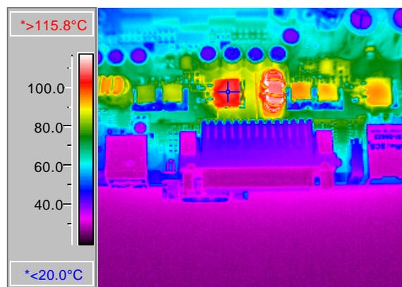
Fig. 6: Infrared camera photograph, existing solution,  $f_{sw}=220KHz$ ,  $I_{out}=40A$ : max. case 106.7°C, max. lead 90.4°C.
