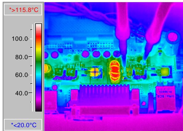
Fig 5: Infrared camera photograph, IRFR3704 with two IRFR3711,  $f_{sw}=220KHz$ ,  $I_{out}=40A$ : max. case 94.2°C, max. lead 81.2°C.
