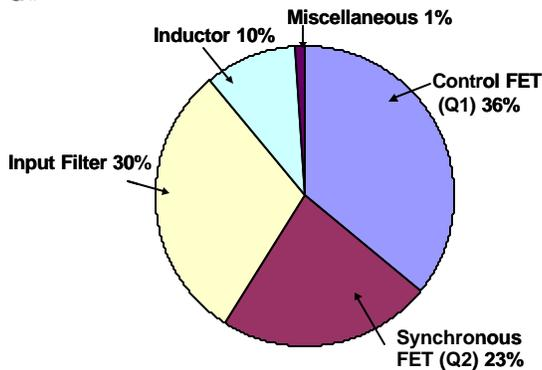
Fig. 2. Power Losses Of A Buck Converter; 12V<sub>IN</sub>, sub-2V<sub>OUT</sub> 300 kHz
