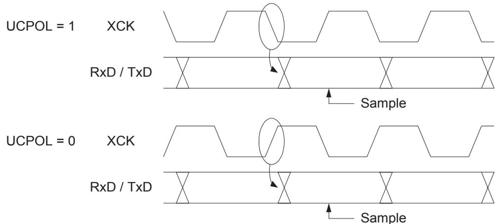
The UCPOL bit UCRSC selects which XCK clock edge is used for data sampling and which is used for data change. As Figure 81 shows, when UCPOL is zero the data will be changed at rising XCK edge and sampled at falling XCK edge. If UCPOL is set, the data will be changed at falling XCK edge and sampled at rising XCK edge.
