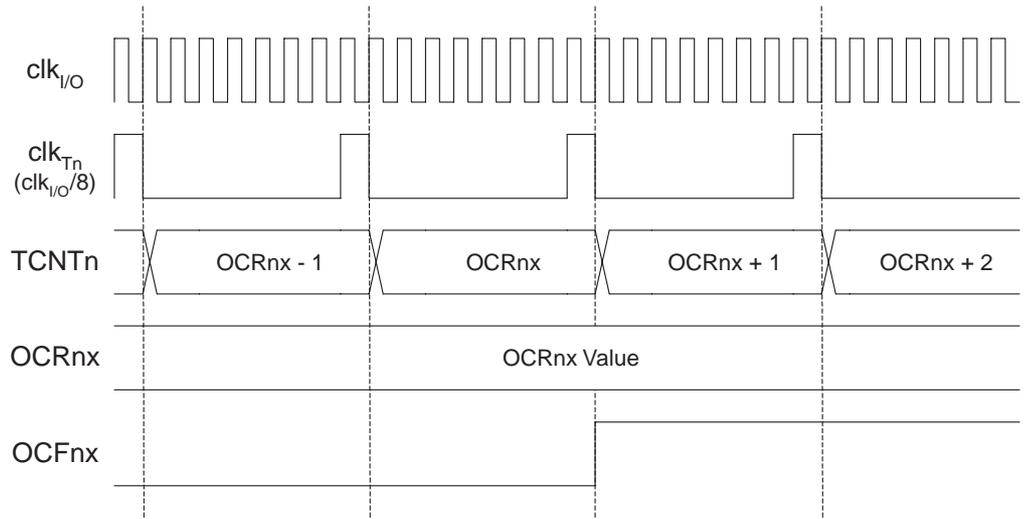
Figure 57 shows the count sequence close to TOP in various modes. When using phase and frequency correct PWM mode the OCRnx Register is updated at BOTTOM. The timing diagrams will be the same, but TOP should be replaced by BOTTOM, TOP-1 by BOTTOM+1 and so on. The same renaming applies for modes that set the TOVn flag at BOTTOM.
