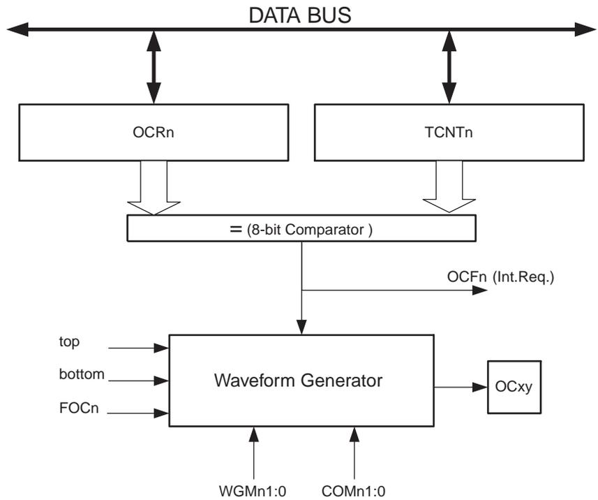
The OCR0 Register is double buffered when using any of the Pulse Width Modulation (PWM) modes. For the normal and Clear Timer on Compare (CTC) modes of operation, the double buffering is disabled. The double buffering synchronizes the update of the OCR0 Compare Register to either top or bottom of the counting sequence. The synchronization prevents the occurrence of odd-length, non-symmetrical PWM pulses, thereby making the output glitch-free.
