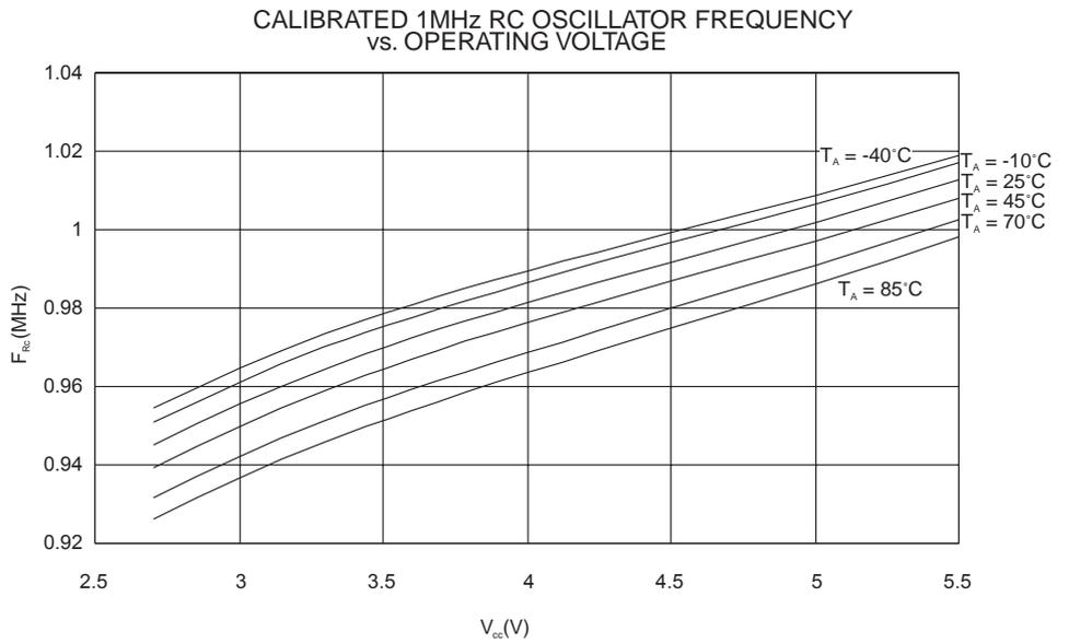
**Figure 197.** RC Oscillator Frequency vs Temperature (the devices are calibrated to 2 MHz at  $V_{cc} = 5V$ ,  $T=25c$ )
