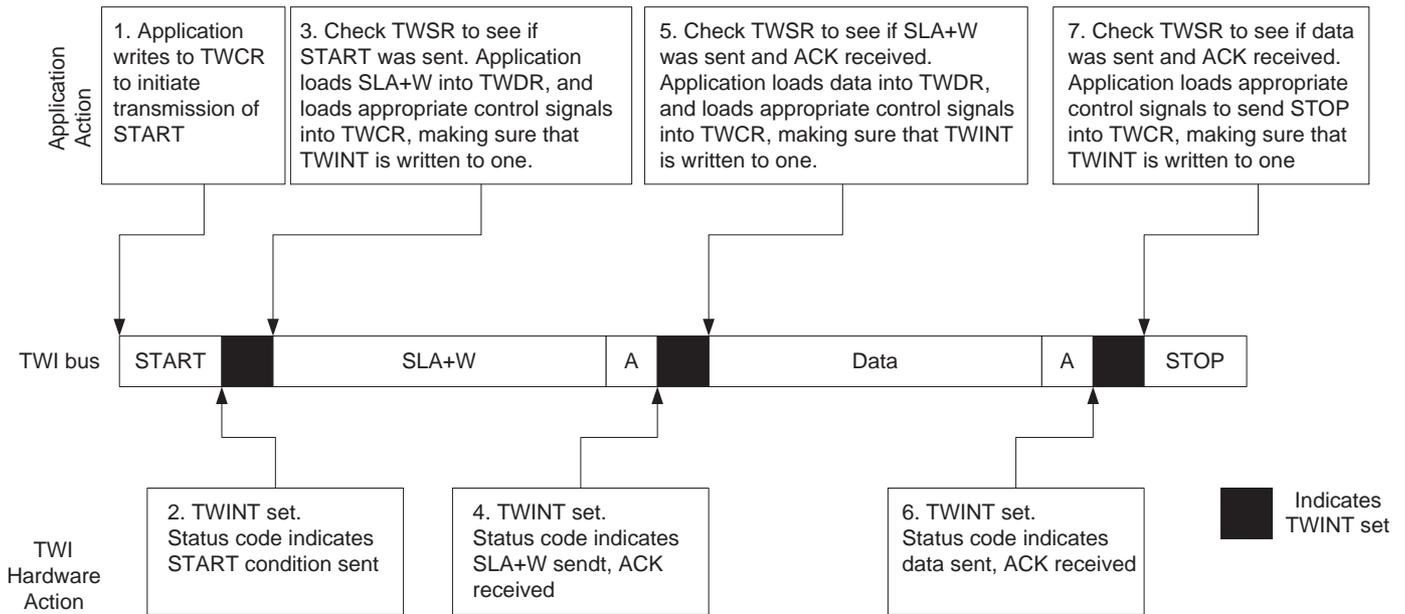
1. The first step in a TWI transmission is to transmit a START condition. This is done by writing a specific value into TWCR, instructing the TWI hardware to transmit a START condition. Which value to write is described later on. However, it is important that the TWINT bit is set in the value written. Writing a one to TWINT clears the flag. The TWI will not start any operation as long as the
