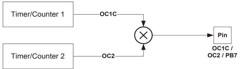
When the modulator is enabled, the two output compare channels are modulated together as shown in the block diagram (Figure 72).
