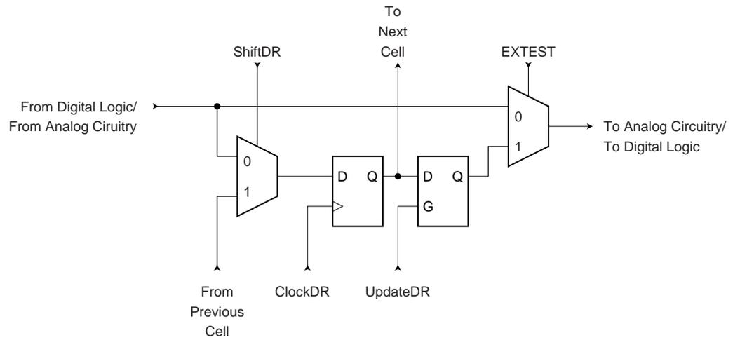
**Table 104.** Boundary-scan Signals for the Analog Comparator
