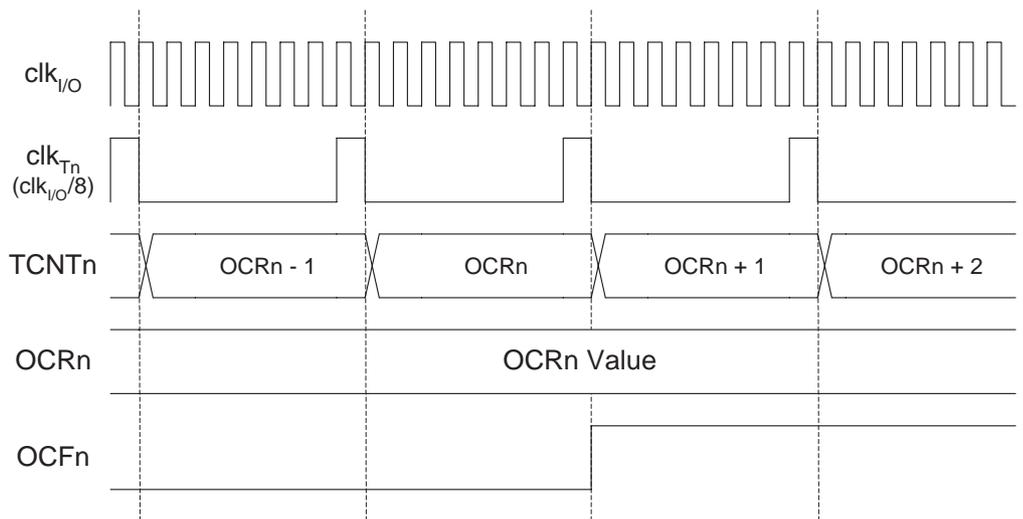
Figure 44 shows the setting of OCF0 and the clearing of TCNT0 in CTC mode.
