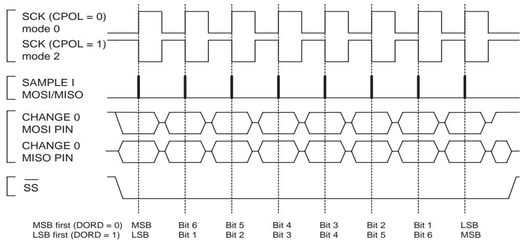
**Figure 78.** SPI Transfer Format with CPHA = 1
