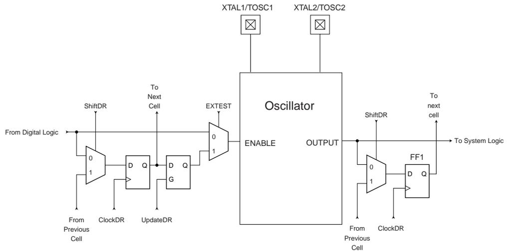
Table 103 summarizes the scan registers for the external clock pin XTAL1, oscillators with XTAL1/XTAL2 connections as well as 32 kHz Timer Oscillator.
