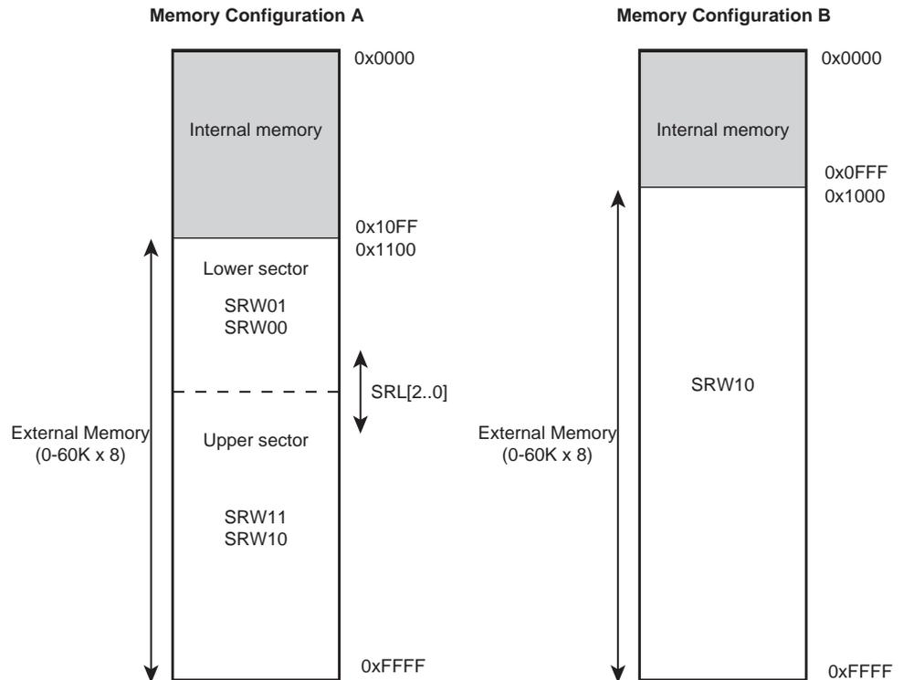
Note: ATmega128 in non ATmega103 compatibility mode: Memory Configuration A is available (Memory Configuration B N/A)
