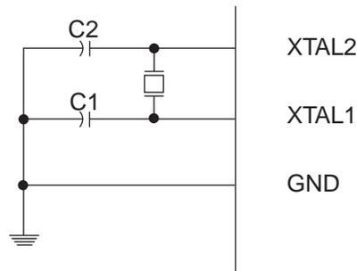
The Oscillator can operate in three different modes, each optimized for a specific frequency range. The operating mode is selected by the fuses CKSEL3..1 as shown in Table 8.
