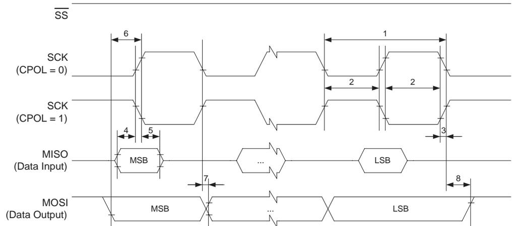
**Figure 155. SPI Interface Timing Requirements (Slave Mode)**
