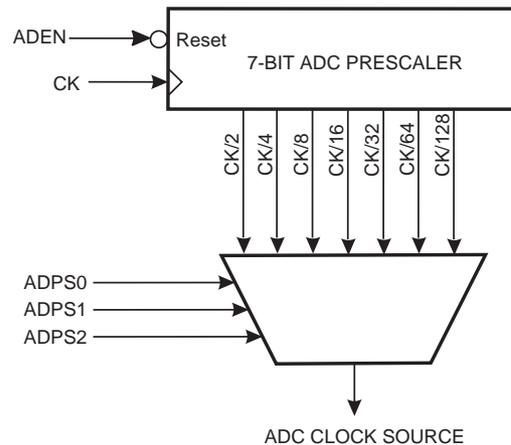
By default, the successive approximation circuitry requires an input clock frequency between 50 kHz and 200 kHz to get maximum resolution. If a lower resolution than 10 bits is needed, the input clock frequency to the ADC can be higher than 200 kHz to get a higher sample rate. Alternatively, setting the ADHSM bit in SFIOR allows an increased ADC clock frequency at the expense of higher power consumption.
