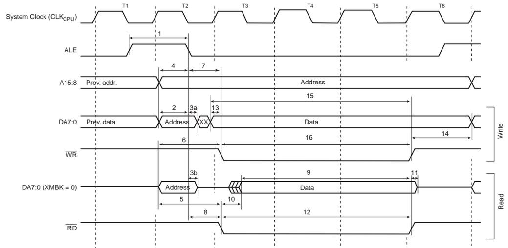
**Figure 159. External Memory Timing (SRWn1 = 1, SRWn0 = 1)<sup>(1)</sup>**
