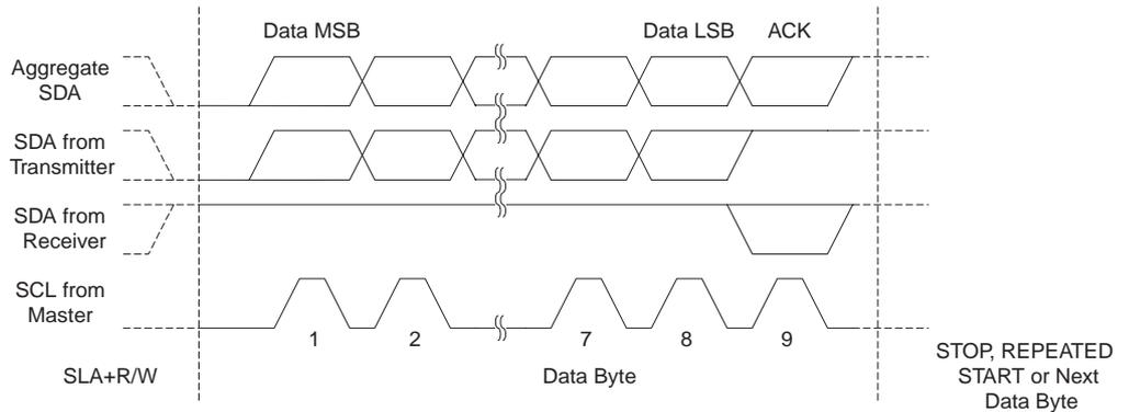
**Combining Address and Data Packets Into a Transmission**
