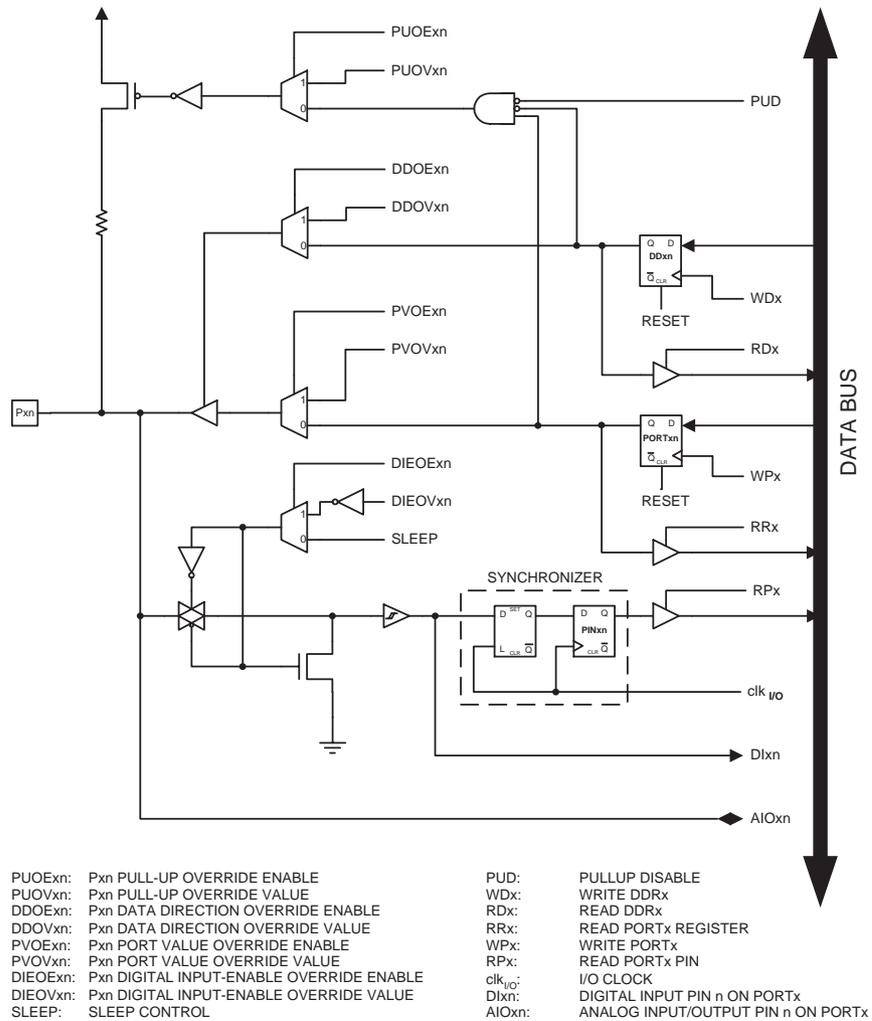
Note: 1. WP<sub>x</sub>, WD<sub>x</sub>, RL<sub>x</sub>, RP<sub>x</sub>, and RD<sub>x</sub> are common to all pins within the same port. clk<sub>I/O</sub>, SLEEP, and PUD are common to all ports. All other signals are unique for each pin.
