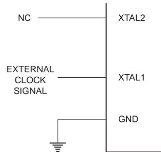
When this clock source is selected, start-up times are determined by the SUT fuses as shown in Table 16.
