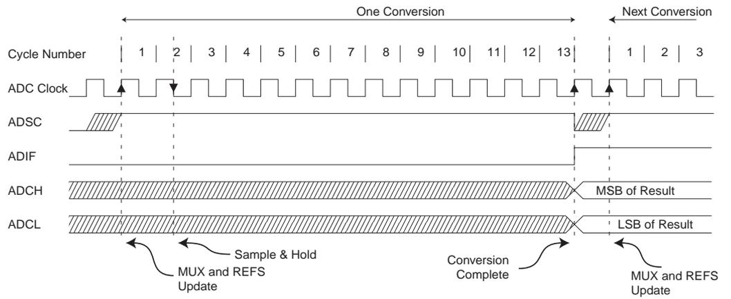
**Figure 112. ADC Timing Diagram, Free Running Conversion**
