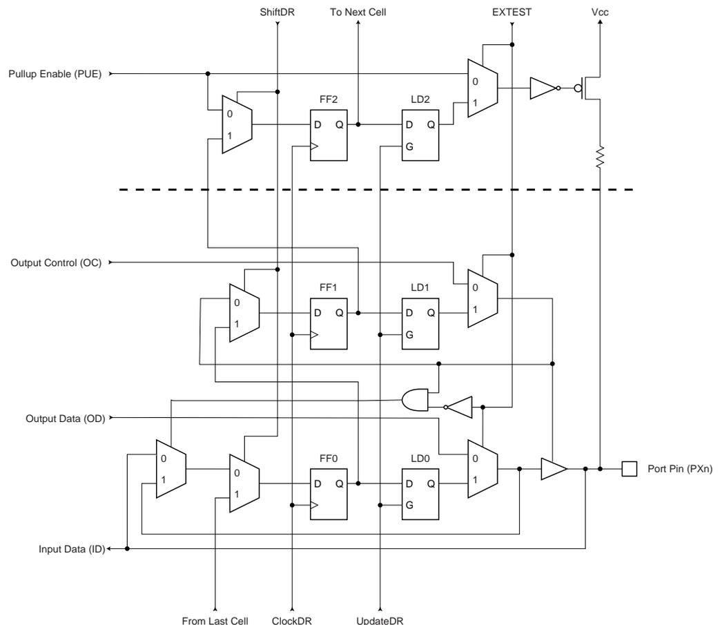
**Figure 125. General Port Pin Schematic diagram**
