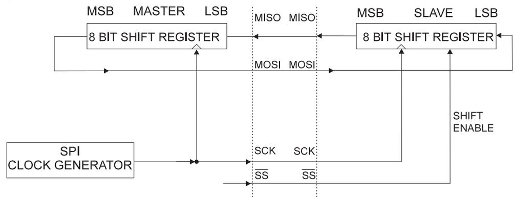
The system is single buffered in the transmit direction and double buffered in the receive direction. This means that bytes to be transmitted cannot be written to the SPI Data Register before the entire shift cycle is completed. When receiving data, however, a received character must be read from the SPI Data Register before the next character has been completely shifted in. Otherwise, the first byte is lost.
