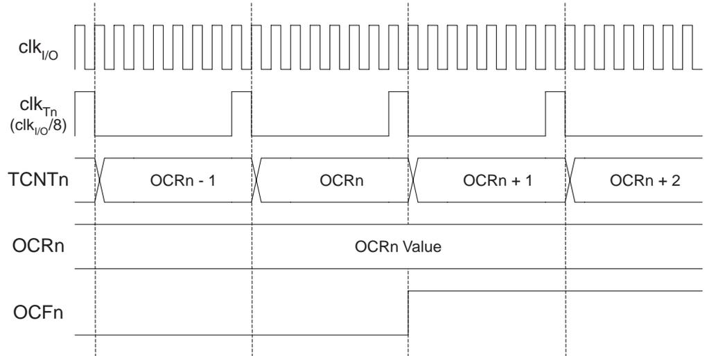
Figure 71 shows the setting of OCF2 and the clearing of TCNT2 in CTC mode.
