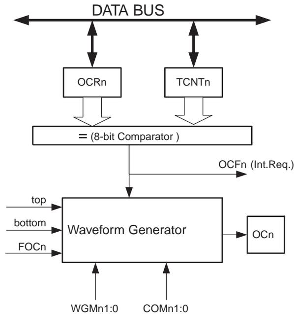
The OCR2 Register is double buffered when using any of the pulse width modulation (PWM) modes. For the normal and Clear Timer on Compare (CTC) modes of operation, the double buffering is disabled. The double buffering synchronizes the update of the OCR2 Compare Register to either top or bottom of the counting sequence. The synchronization prevents the occurrence of odd-length, non-symmetrical PWM pulses, thereby making the output glitch-free.
