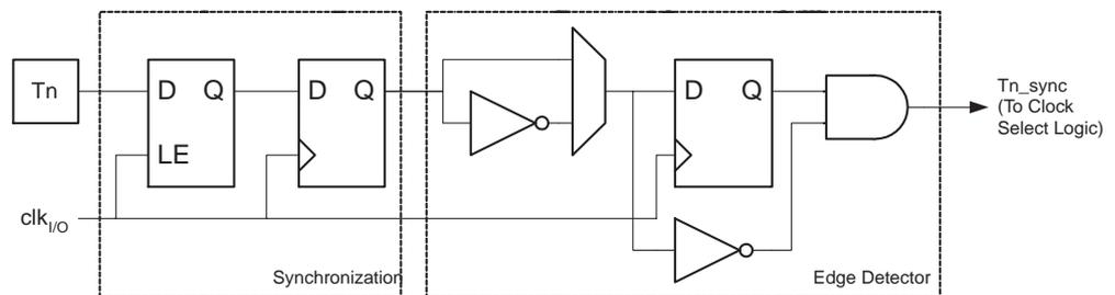
The synchronization and edge detector logic introduces a delay of 2.5 to 3.5 system clock cycles from an edge has been applied to the Tn pin to the counter is updated.
