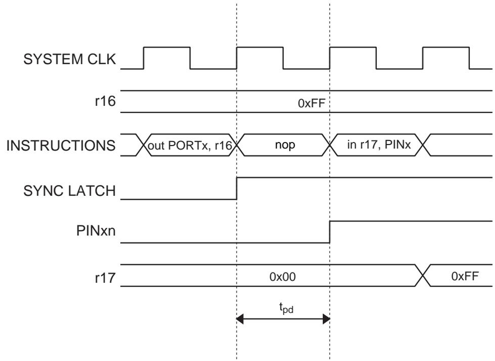
The following code example shows how to set port B pins 0 and 1 high, 2 and 3 low, and define the port pins from 4 to 7 as input with pull-ups assigned to port pins 6 and 7. The resulting pin values are read back again, but as previously discussed, a *nop* instruction is included to be able to read back the value recently assigned to some of the pins.
