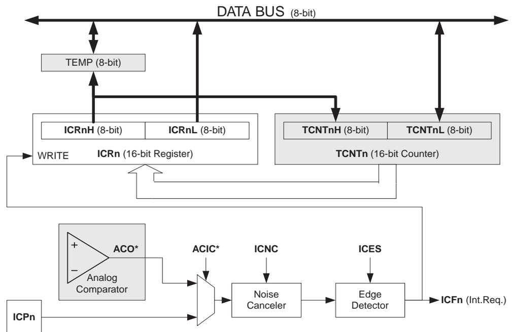
Note: The Analog Comparator Output (ACO) can only trigger the Timer/Counter1 ICP – not Timer/Counter3.
