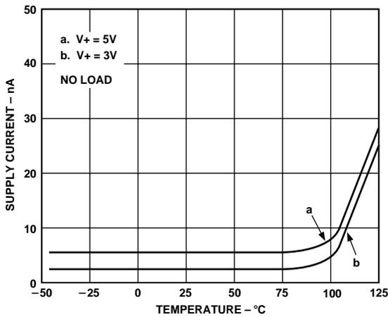
Figure 9. Supply Current vs. Temperature (Shutdown = 0 V)
