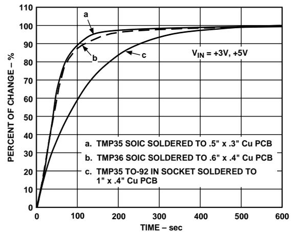
Figure 13. Thermal Response Time in Still Air
