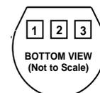
PIN 1 - +Vs, PIN 2 - VOUT, PIN 3 - GND
