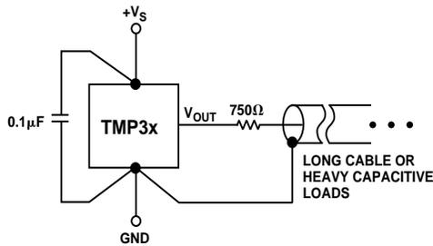
Figure 27. Driving Long Cables or Heavy Capacitive Loads
