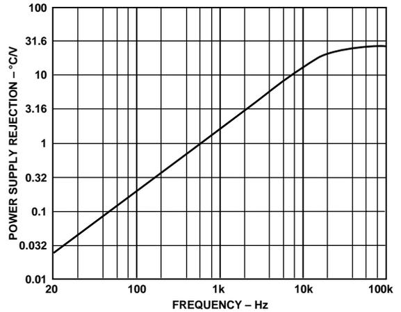
Figure 5. Power Supply Rejection vs. Frequency
