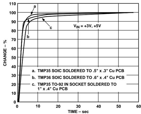
Figure 15. Thermal Response Time in Stirred Oil Bath
