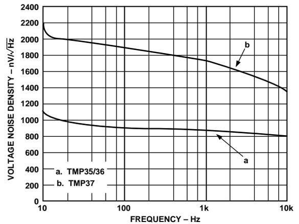
Figure 17. Voltage Noise Spectral Density vs. Frequency
