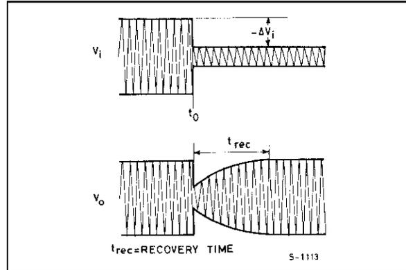
The recovery time ( $T_{rec}$ ) is defined as the time between the instant  $T_0$  and the instant in which the output signal returns to the nominal level.
