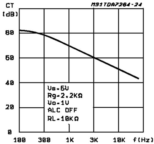
Figure 14: Crosstalk vs. Frequency (ALC = Off)
