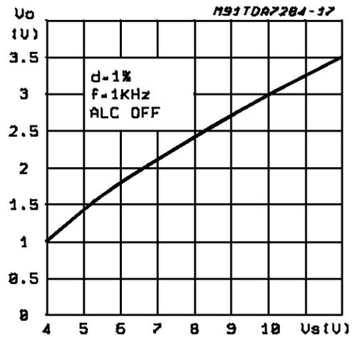
Figure 8: Output Voltage vs. Input Voltage
