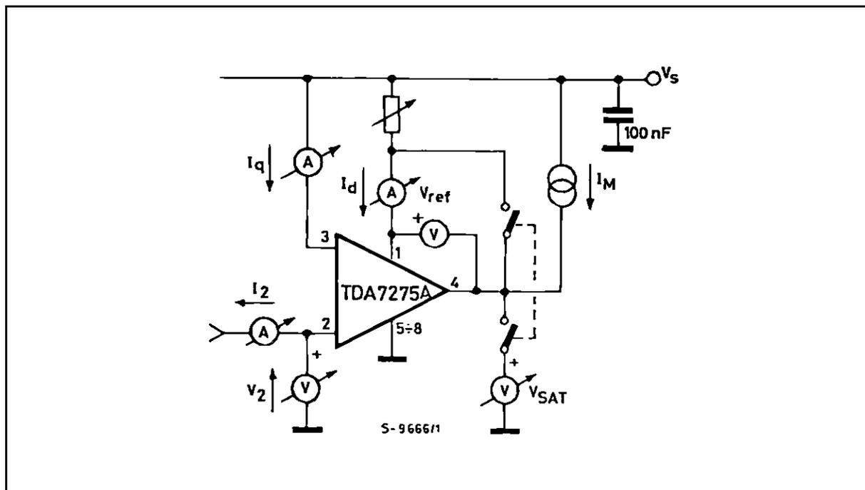
Figure 2 : Application Circuit.
