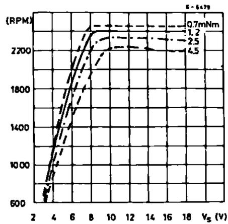
**Figure 5 :** Speed Variation vs. Torque ( $V_S = 12V$ ).
