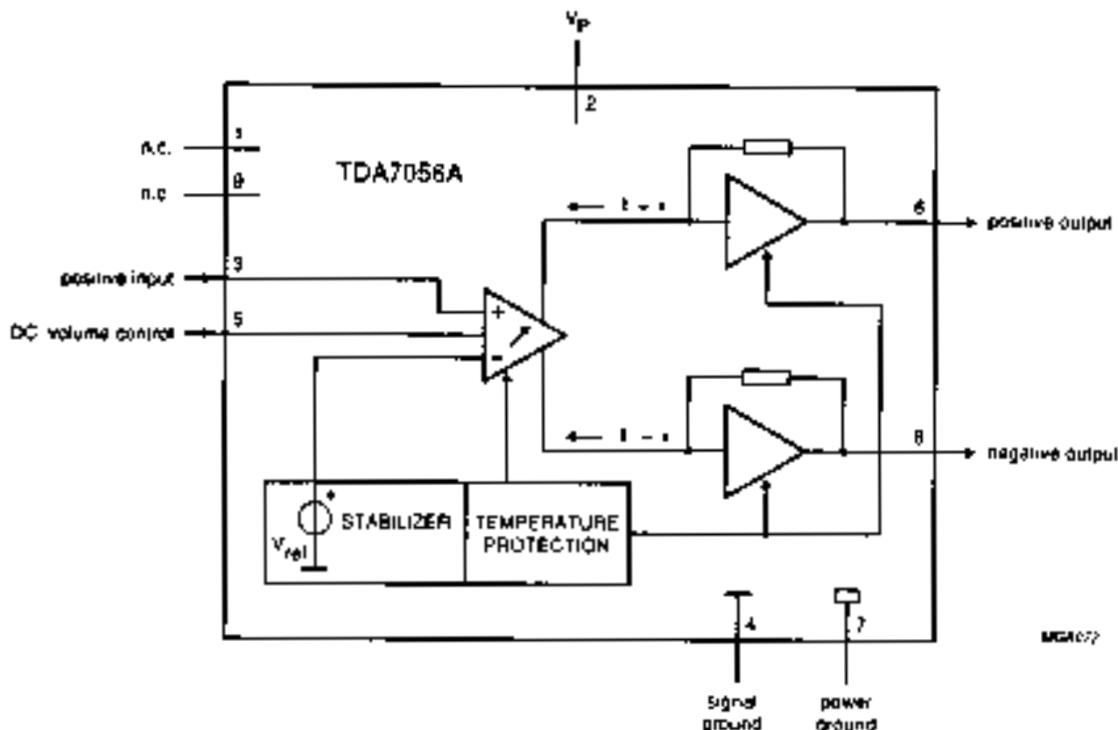
Fig.1 Block diagram.
