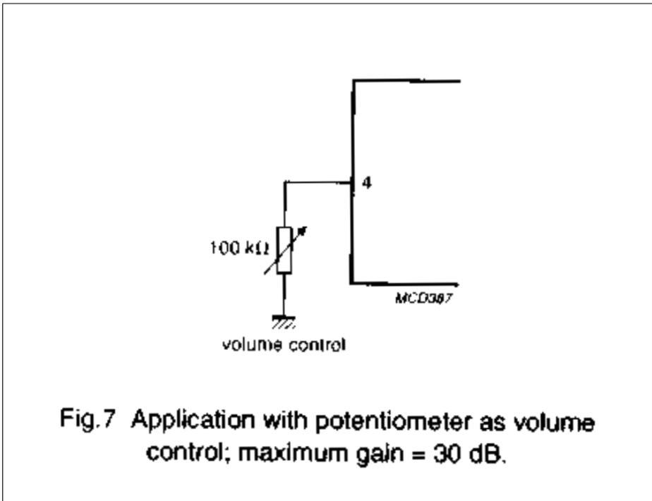
**Fig.7 Application with potentiometer as volume control; maximum gain = 30 dB.**
