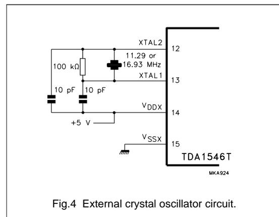
Fig.4 External crystal oscillator circuit.
