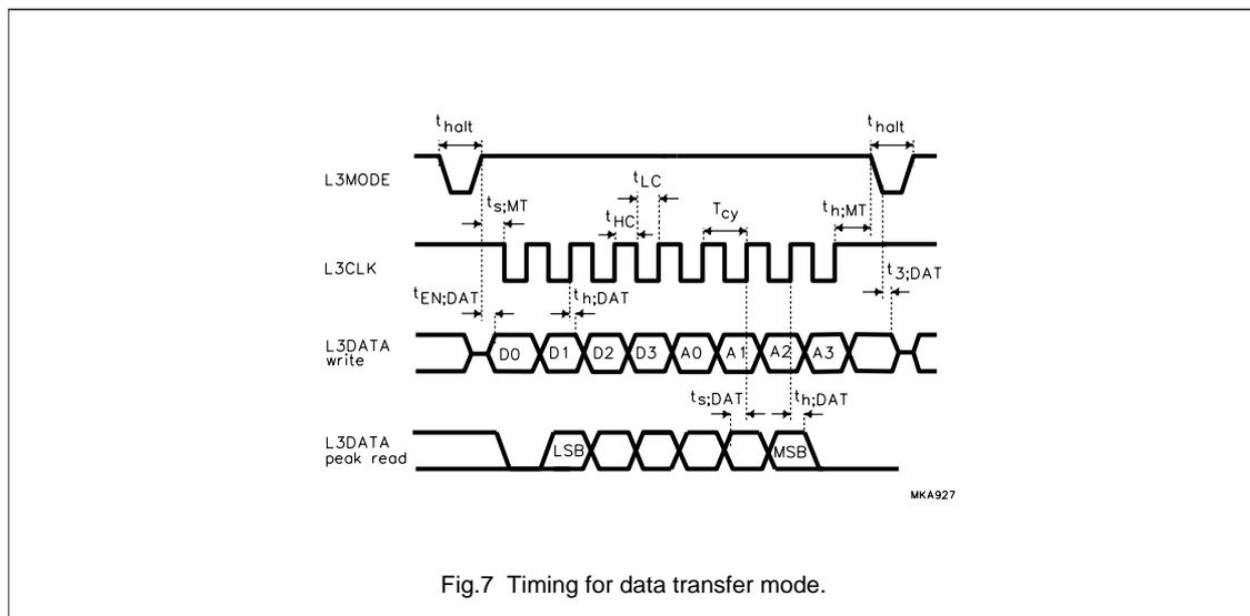
Fig.7 Timing for data transfer mode.
