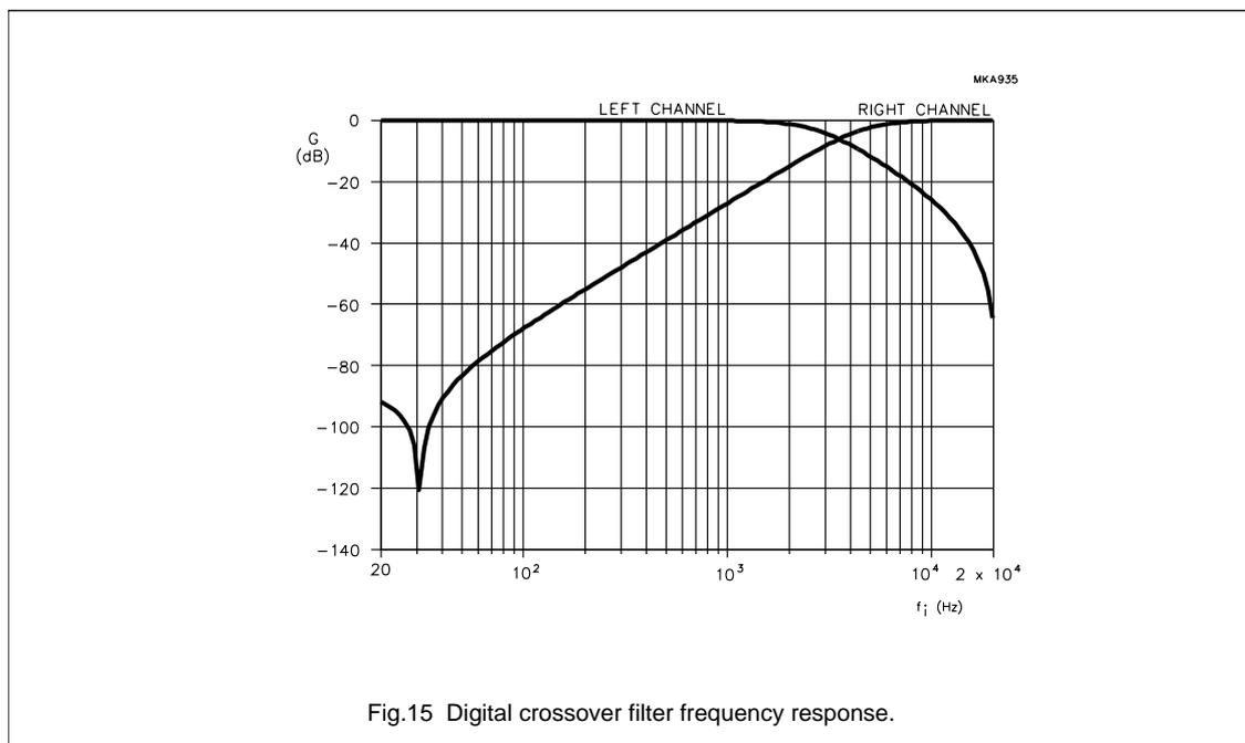
Fig.15 Digital crossover filter frequency response.
