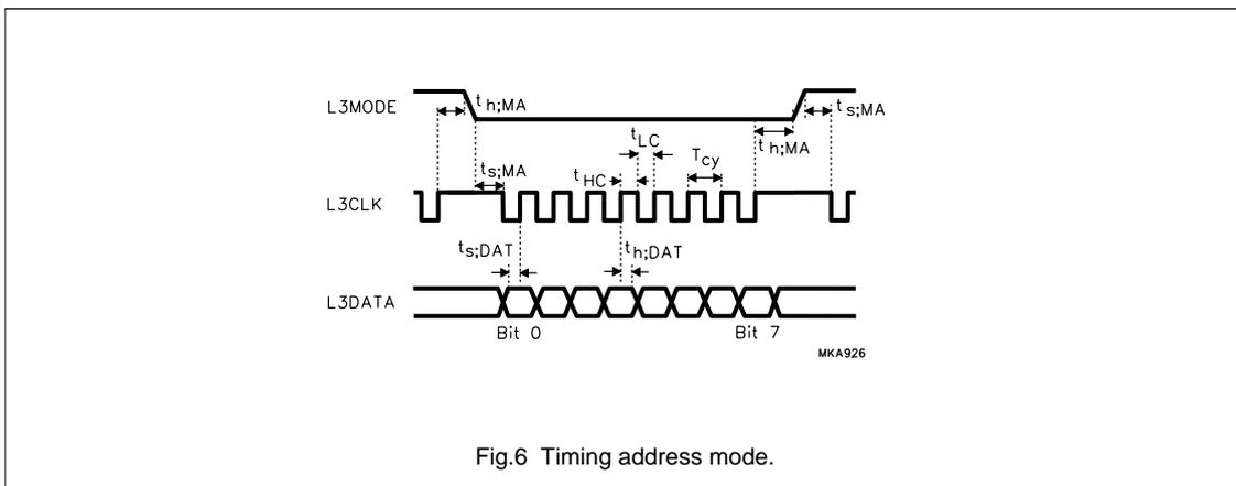
Fig.6 Timing address mode.
