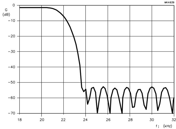
Fig.19 Digital filter transition band.
