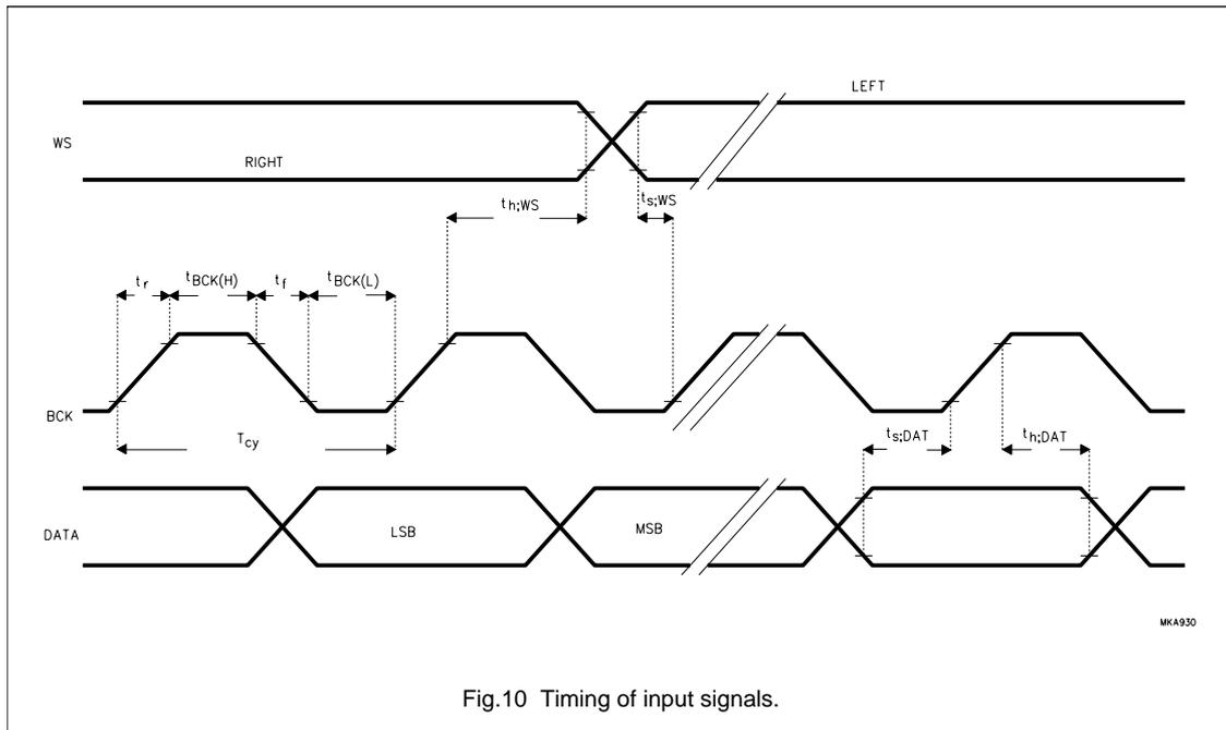
Fig.10 Timing of input signals.
