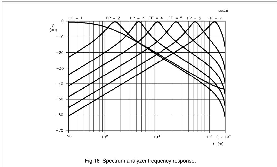
Fig.16 Spectrum analyzer frequency response.
