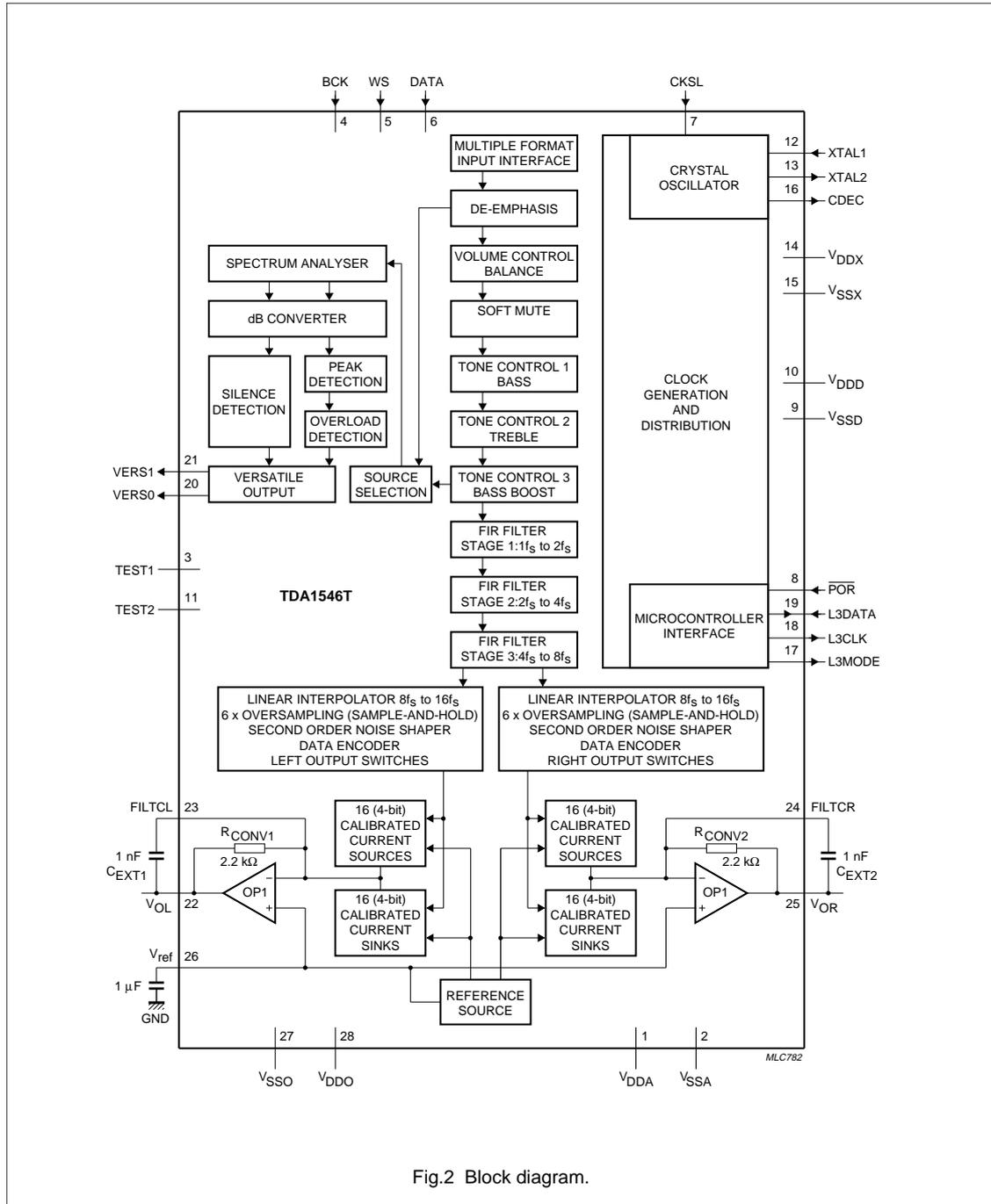
Fig.2 Block diagram.
