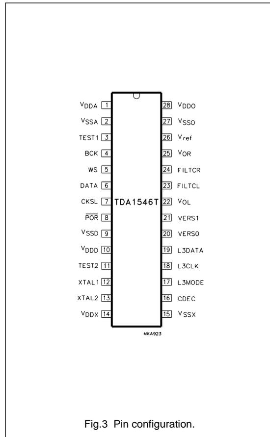
Fig.3 Pin configuration.
