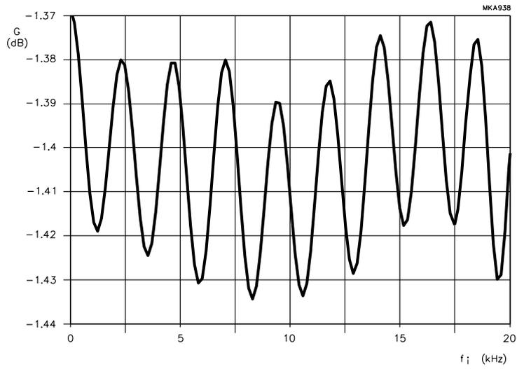
Fig.18 Digital filter pass band ripple.
