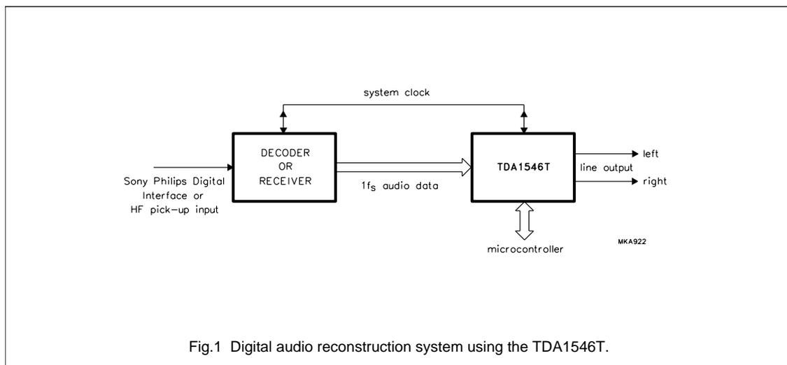
Fig.1 Digital audio reconstruction system using the TDA1546T.
