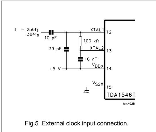
Fig.5 External clock input connection.
