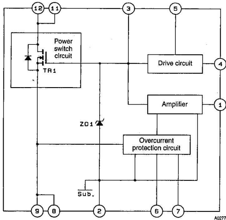
The back surface of the IC is not an insulator, and is effectively at pin 2 potential.
