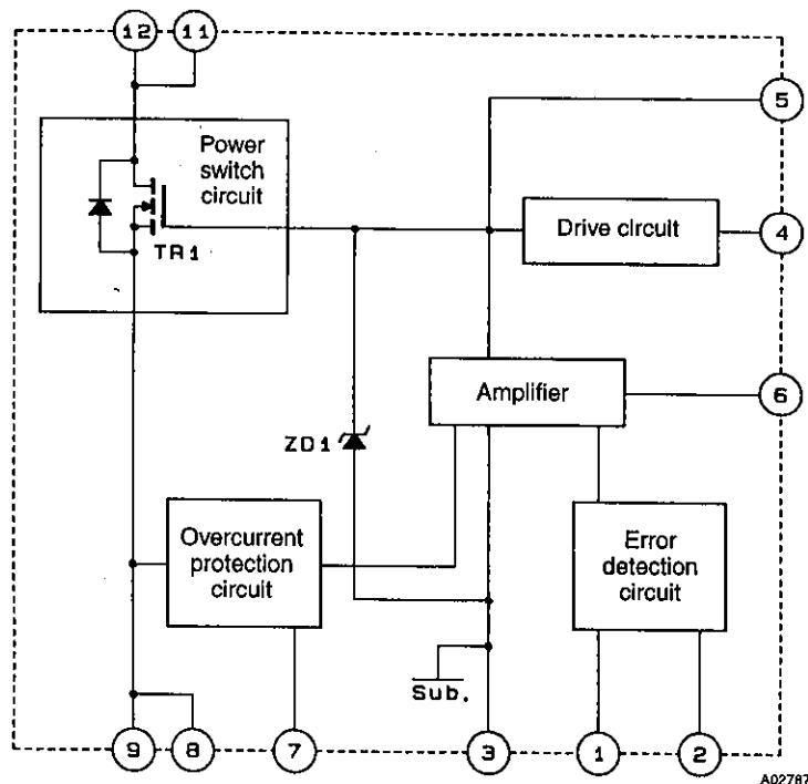
The back surface of the IC is not an insulator, and is effectively at pin 3 potential.
