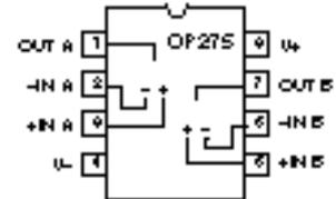
Improved dc performance is also provided with bias and offset currents greatly reduced over purely bipolar designs. Input offset voltage is guaranteed at 1 mV and is typically less than 200  $\mu\text{V}$ . This allows the OP275 to be used in many dc coupled or summing applications without the need for special selections or the added noise of additional offset adjustment circuitry.
