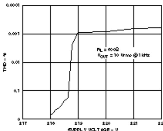
Figure 5. THD + Noise vs. Supply Voltage
