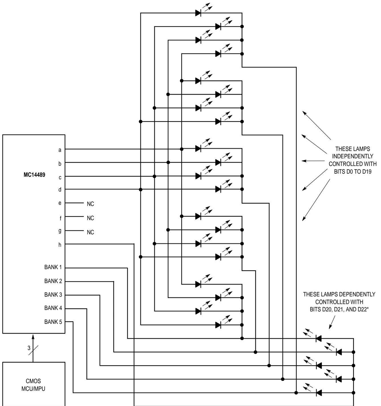
\* If required, this group of lamps can be independently controlled. To accomplish independent control, only connect lamps to BANK 1 and BANK 2 for output h (two lamps). Then, use bits D20, D21, and D22 for control of these two lamps.
