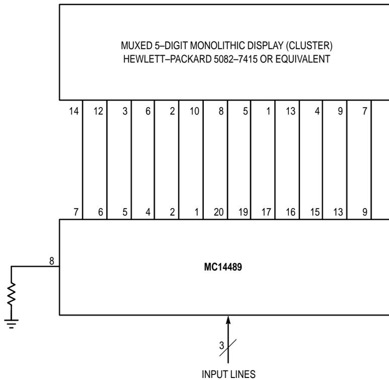
**Figure 19. Compact Display System with Three Components**
