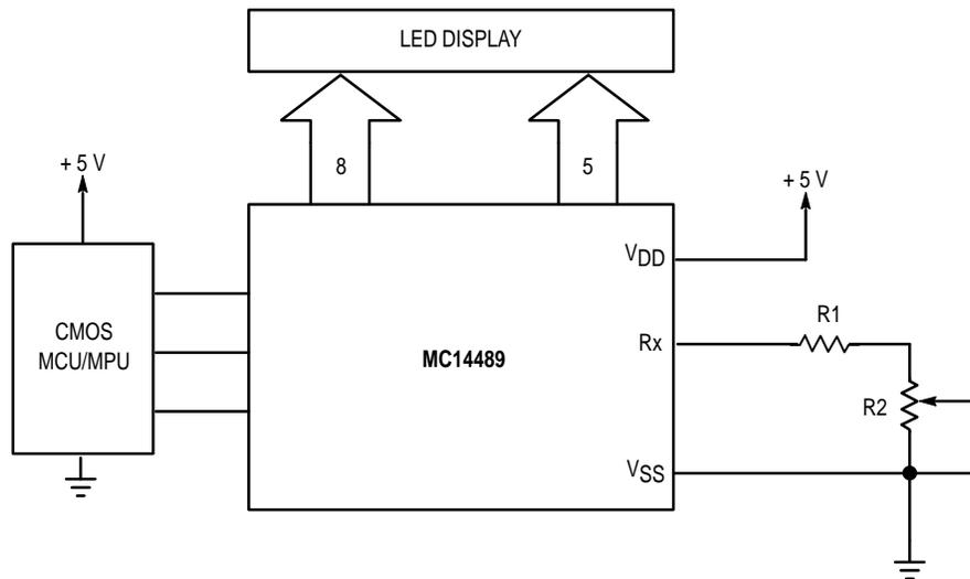
NOTE: R1 limits the maximum current to avoid damaging the display and/or the MC14489 due to overheating. See the Thermal Considerations section. An 1/8 watt resistor may be used for R1. R2 is a 1 kΩ or 5 kΩ potentiometer ( $\geq 1/8$  watt). R2 may be a light-sensitive resistor.
