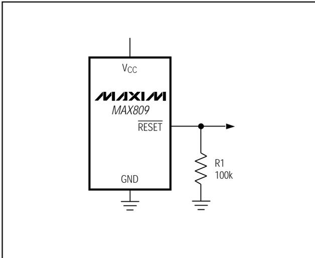
Figure 2.  $\overline{\text{RESET}}$  Valid to  $V_{CC}$  = Ground Circuit
