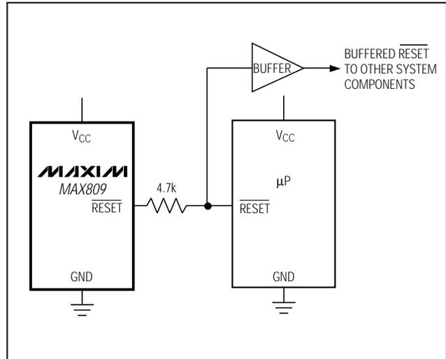
Figure 3. Interfacing to  $\mu\text{Ps}$  with Bidirectional Reset I/O
