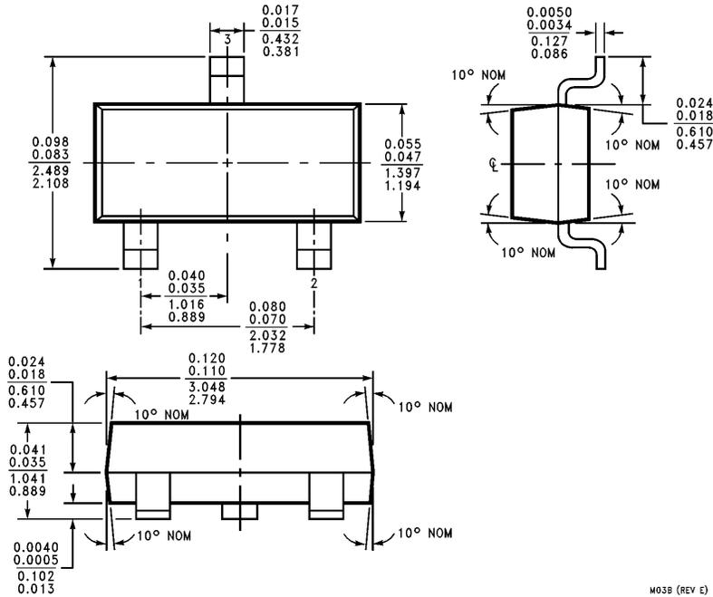
**SOT-23 Molded Small Outline Transistor Package (M3)**
