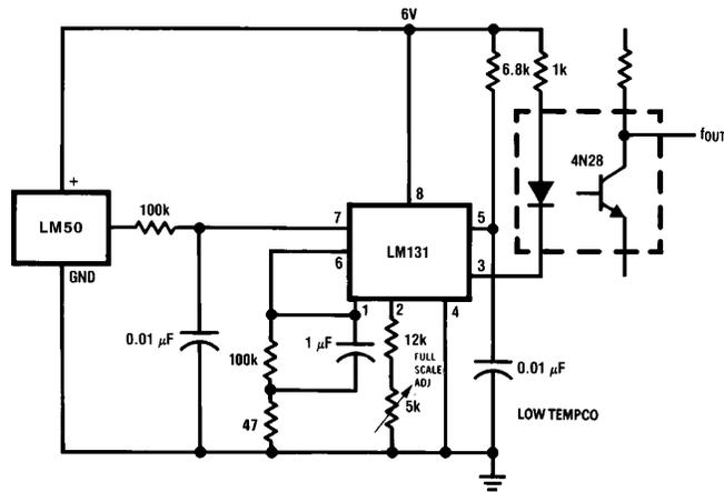
FIGURE 9. LM50 With Voltage-To-Frequency Converter And Isolated Output
