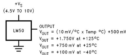
FIGURE 1. Full-Range Centigrade Temperature Sensor ( $-40^{\circ}\text{C}$  to  $+125^{\circ}\text{C}$ )
