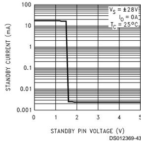
**Supply Current ( $I_{EE}$ ) vs Standby Pin Voltage**
