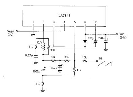
Unit (resistance:  $\Omega$ , capacitance: F)
