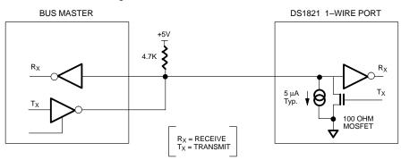
The idle state for the 1–Wire bus is high. If for any reason a transaction needs to be suspended, the bus MUST be left in the idle state if the transaction is to resume. Infinite recovery time can occur between bits so long as the 1–Wire bus is in the inactive (high) state during the recovery period. If this does not occur and the bus is left low for more than 480  $\mu s$ , all components on the bus will be reset.
