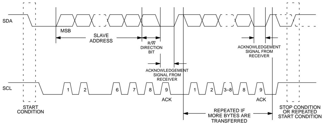
Figure 4 details how data transfer is accomplished on the two-wire bus. Depending upon the state of the R/W bit, two types of data transfer are possible:
