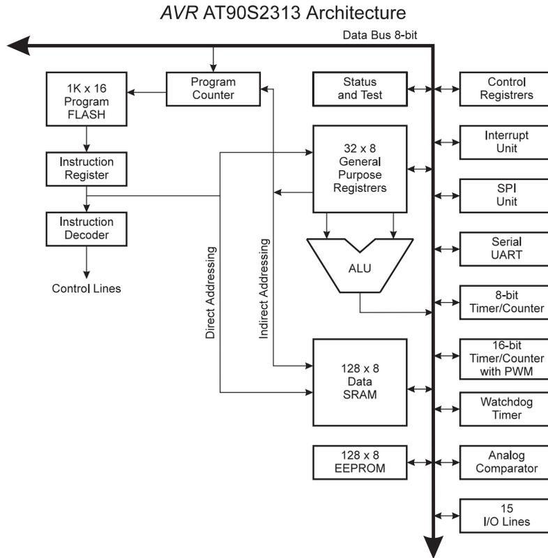
**Figure 2.** The AT90S2313 AVR Enhanced RISC Architecture
