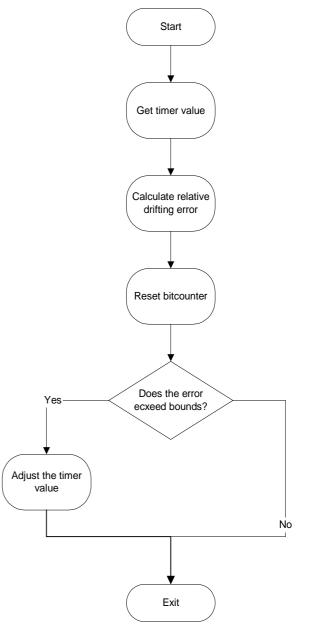
The receiving algorithm should be operated by a timer, as for the oversampling case. But to adjust the timer and avoid errors due to drifting in sampling time, the edge sensing algorithm should be run as a routine for the external interrupt source. This means that the incoming bitstream should be tracked to a pin on the MCU that can give interrupt from a change in the logical value of a signal.
