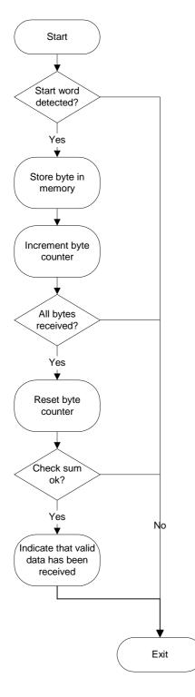
This routine must be run each time the UART has received a whole byte. In most microcontrollers with hardware implemented UART, an interrupt is send to the MCU each time a complete byte is received. Detection of start word can be done by setting a bit in a dedicated control register.
