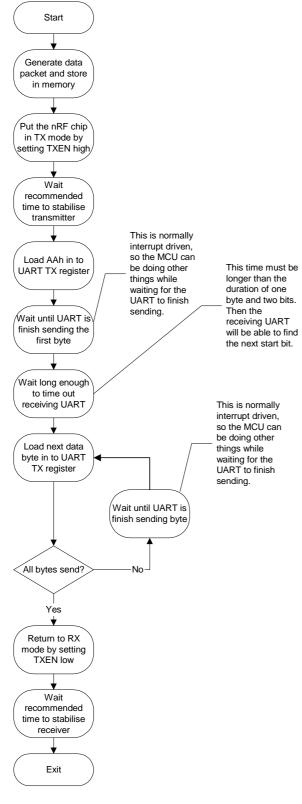
This flowchart shows how to send a data packet via hardware UART. To implement this routine you should consider use of the UARTs ability to make interrupts to the MCU. The parts of this routine that requires waiting for the UART to finish, should be implemented to run as an interrupt routine.
