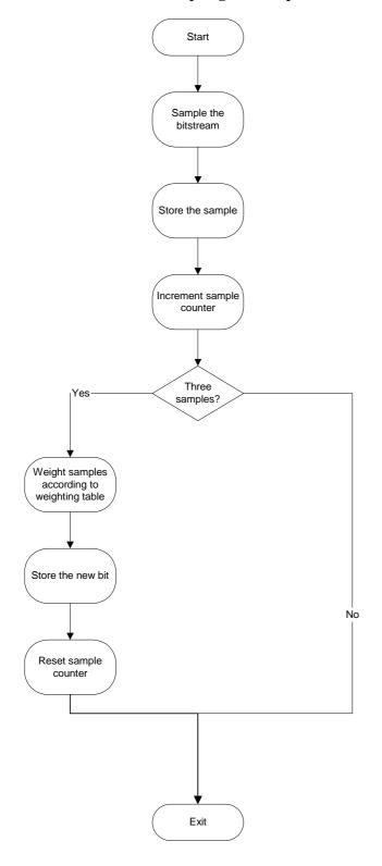
This algorithm must be implemented as a timer overflow interrupt routine in a MCU. Then the timer should be set to time out three times per bit periode. It is important that this routine is implemented as short and efficient as possible, because even if a MCU runs at 4 MHz cyckle, sampling a 20 kbits/s bit stream three times each bit gives only 66 cycles to handle each sample.
