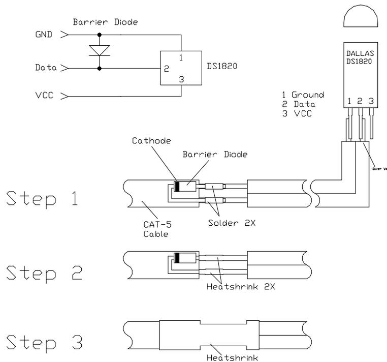
Step 1: Locate the silver and copper wires coming from the probe. Solder a diode across the wires as shown in step 1 above.
