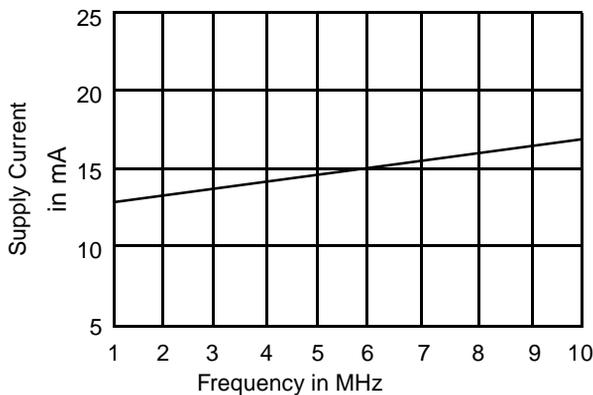
**Figure 1. Typical Supply Current vs. Frequency**
