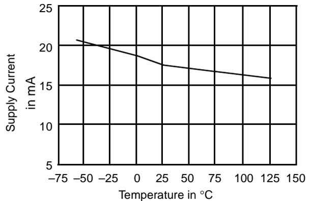
**Figure 2. Typical Supply Current vs. Temperature**
