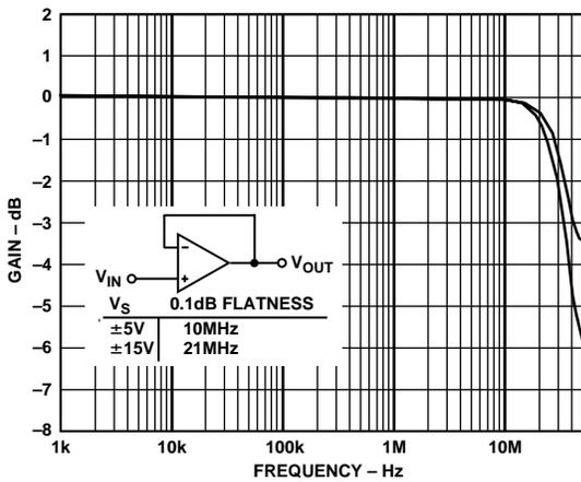
Figure 16. Closed-Loop Gain vs. Frequency, Gain = +1
