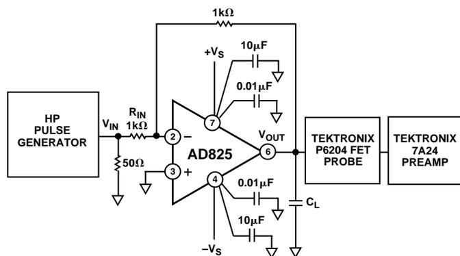
Figure 26a. Inverting Amplifier Driving a Capacitive Load
