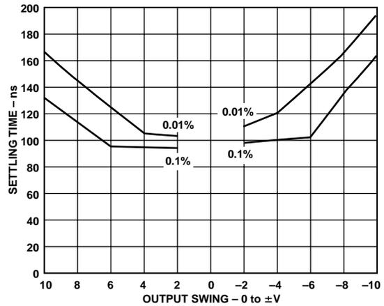
Figure 13. Output Swing and Error vs. Settling Time
