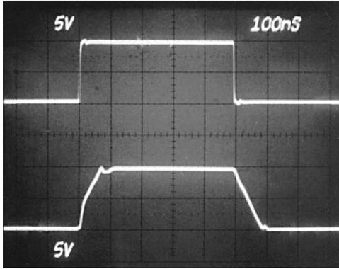
Figure 21. Noninverting Large Signal Pulse Response,  $R_L = 150 \Omega$
