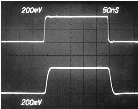
Figure 22. Noninverting Small Signal Pulse Response,  $R_L = 150 \Omega$
