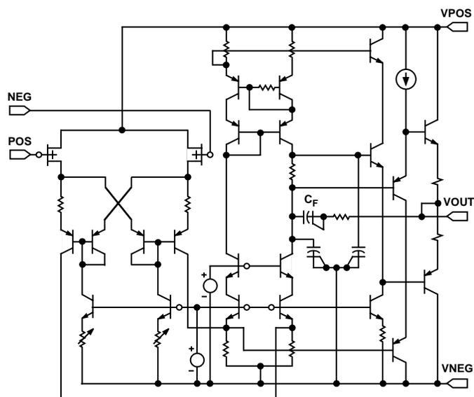
Figure 27. Simplified Schematic
