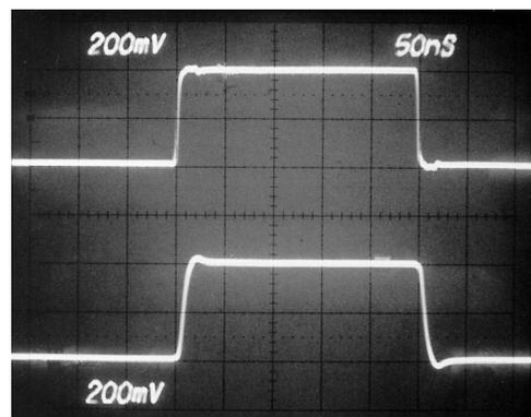
Figure 20. Noninverting Small Signal Pulse Response,  $R_L = 1 \text{ k}\Omega$
