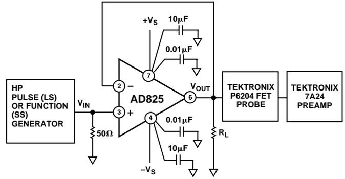
Figure 18. Noninverting Amplifier Connection
