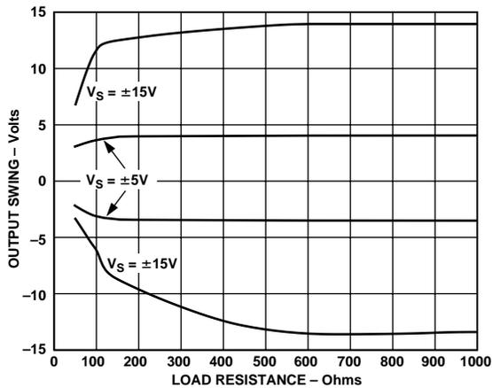
Figure 4. Output Voltage Swing vs. Load Resistance
