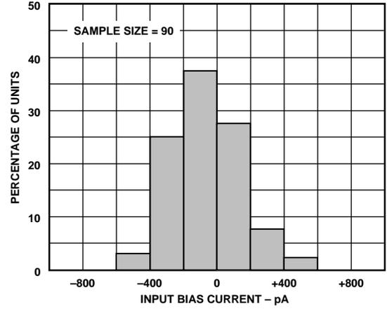
Figure 4. Typical Distribution of Input Bias Current
