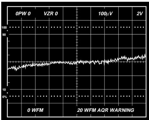
Figure 26. Gain Nonlinearity,  $G = 100$ ,  $R_L = 10 \text{ k}\Omega$ ,  $C_L = 0 \text{ pF}$ . Vertical Scale:  $100 \mu\text{V}/\text{Div} = 100 \text{ ppm}/\text{Div}$  Horizontal Scale:  $2 \text{ Volts}/\text{Div}$
