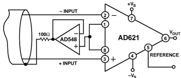
Figure 40. Common-Mode Shield Driver, G = 100
