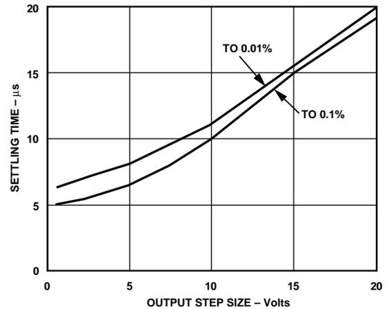
Figure 23. Settling Time vs. Step Size,  $G = 10$
