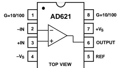
pin strapping. The AD621 is fully specified as a total system, therefore, simplifying the design process.
