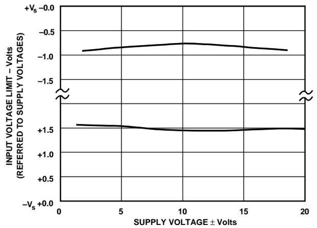
Figure 16. Input Voltage Range vs. Supply Voltage
