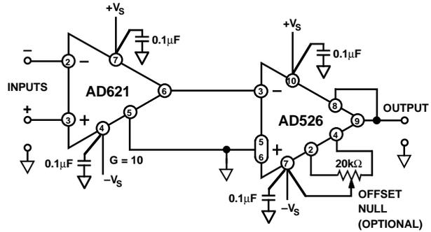
Figure 38. A High Performance Programmable Gain Amplifier
