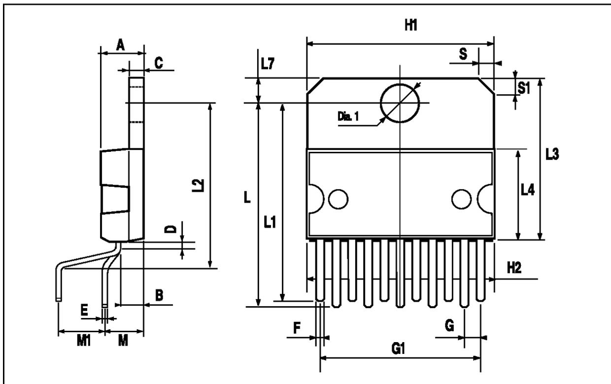
MULTIWATT11 (In line) PACKAGE MECHANICAL DATA
