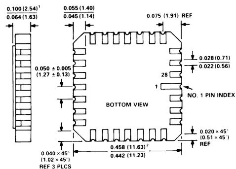
1. THIS DIMENSION CONTROLS THE OVERALL PACKAGE THICKNESS.
