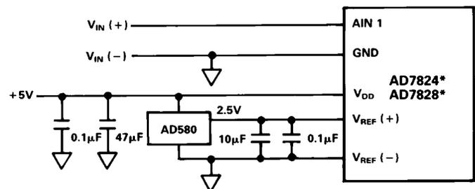
\*ADDITIONAL PINS OMITTED FOR CLARITY, ONLY CHANNEL 1 SHOWN
