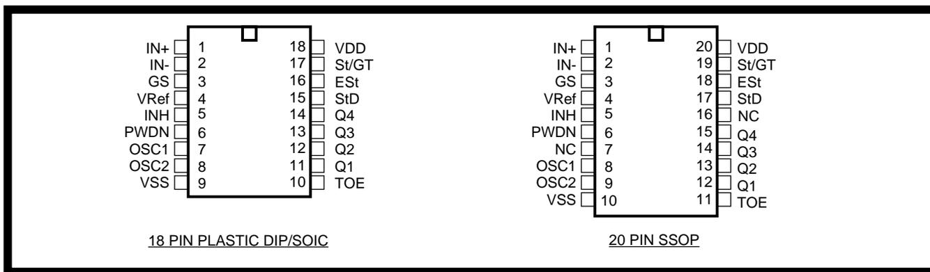
Figure 2 - Pin Connections
