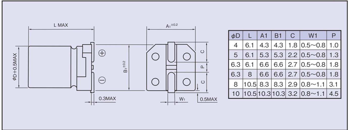
◆ STANDARD SIZE Size φD×L(mm), Rated Ripple Current (mA r.m.s./105°C, 100kHz), Impedance(Ω MAX/20°C, 100kHz)
