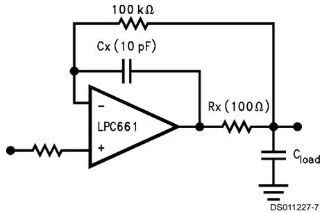
**FIGURE 2. R<sub>x</sub>, C<sub>x</sub> Improve Capacitive Load Tolerance**
