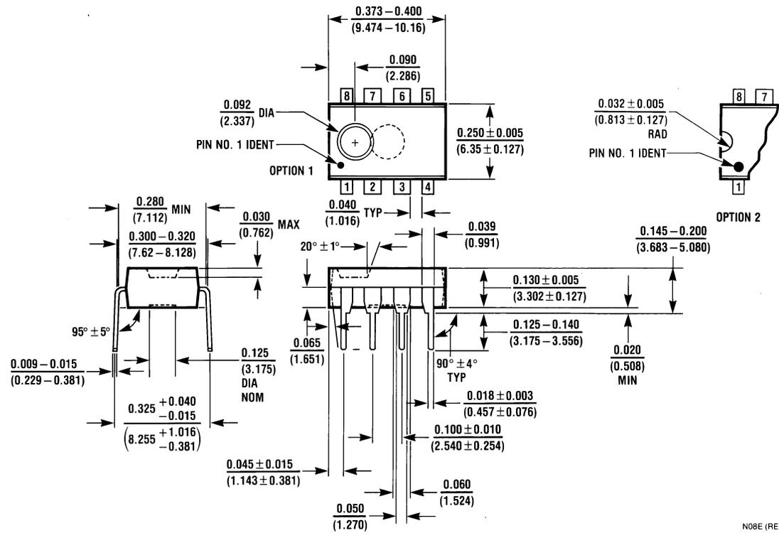
**8-Pin Molded Dual-In-Line Package (N)**
