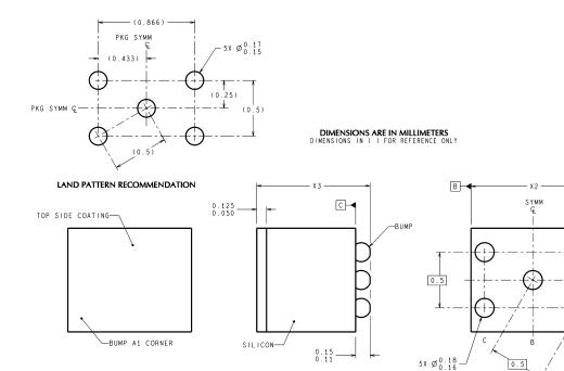
micro SMD, 5 Bump, Package (BPA05) **NS Package Number BPA05DNC** The dimensions for X1, X2 and X3 are as given:
