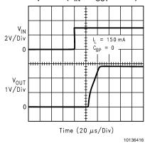
Start Up Time ( $V_{IN} = 4.2V$ )
