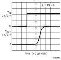
Start Up Time ( $V_{IN} = V_{OUT} + 0.2V$ )
