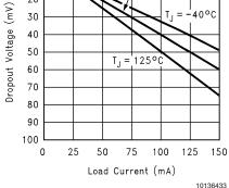
**Dropout Voltage vs Load Current**
