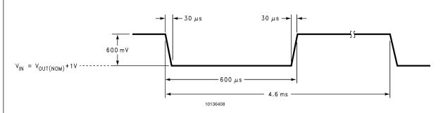
FIGURE 1. Line Transient Input Test Signal
