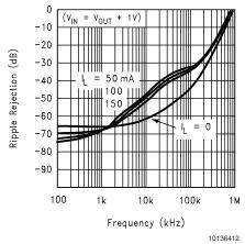
Ripple Rejection (V<sub>IN</sub> = 5.0V)
