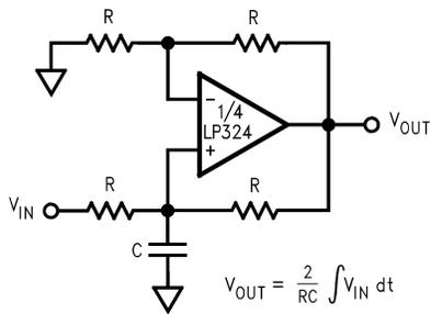
$$V_{OUT} = \frac{2}{RC} \int V_{IN} dt$$
