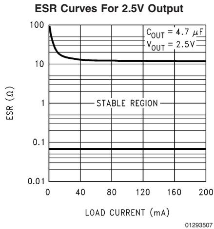
**IMPORTANT:** The output capacitor must maintain its ESR in the stable region over the full operating temperature range of the application to assure stability.
