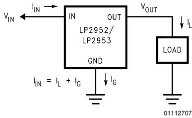
**FIGURE 1.  $P_{TOTAL} = (V_{IN} - V_{OUT}) I_L + (V_{IN}) I_G$
