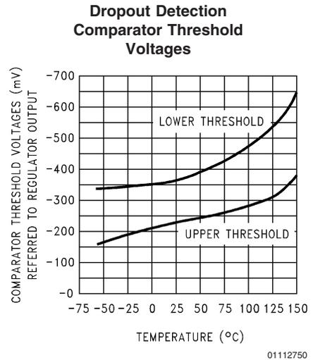
**Typical Performance Characteristics** Unless otherwise specified:  $V_{IN} = 6V$ ,  $I_L = 1\text{ mA}$ ,  $C_L = 2.2\text{ }\mu\text{F}$ ,  $V_{SD} = 3V$ ,  $T_A = 25^\circ\text{C}$ ,  $V_{OUT} = 5V$ . (Continued)
