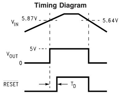
$T_d = (0.28) RC = 28 \text{ ms}$  for components shown.
