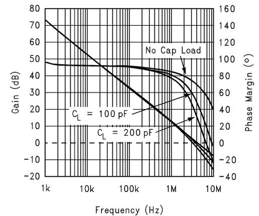
**Typical Performance Characteristics** Unless otherwise specified,  $V_S = +5V$ , single supply,  $T_A = 25^\circ C$ . (Continued)
