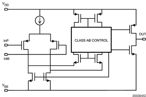
FIGURE 1. Simplified Schematic
