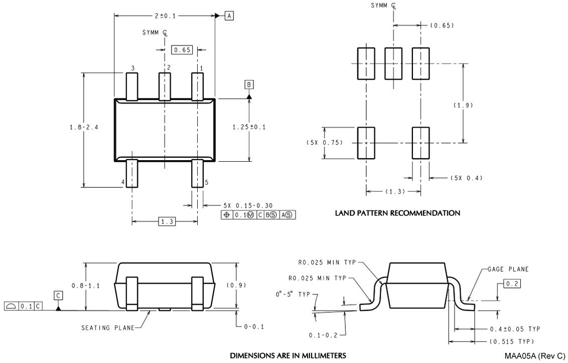
DIMENSIONS ARE IN MILLIMETERS
