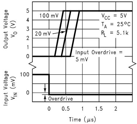
**Typical Performance Characteristics** Unless otherwise specified,  $V_S = +5V$ , single supply,  $T_A = 25^\circ C$  (Continued)
