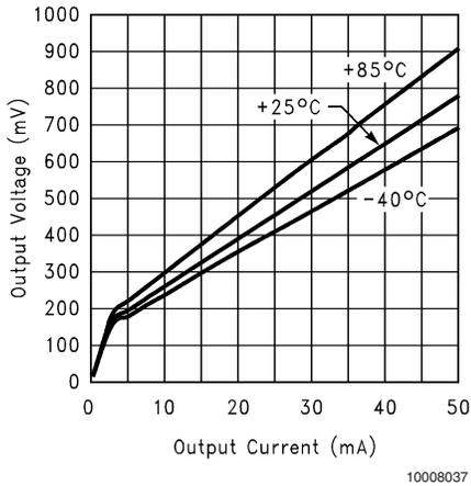
**Output Voltage vs. Output Current at 2.7 Supply**
