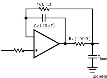
**FIGURE 2. Rx, Cx Improve Capacitive Load Tolerance**
