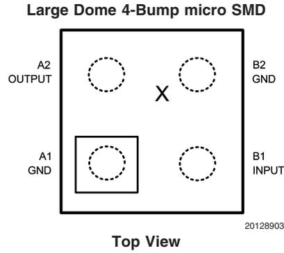
**Note:** - Pin numbers are referenced to package marking text orientation.
