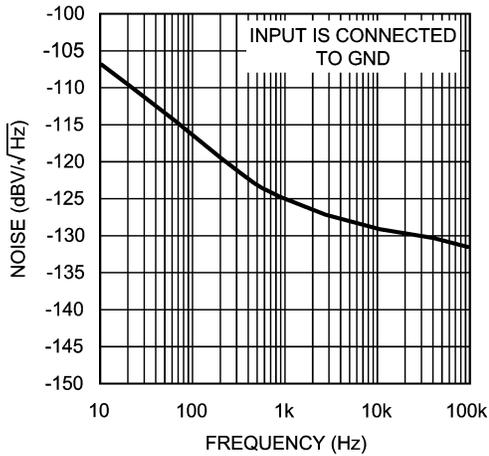
**Output Noise vs. Frequency (LMV1015-25)**
