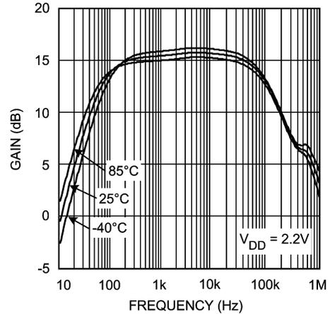
**FIGURE 5. LMV1015-15 Gain vs. Frequency Over Temperature**
