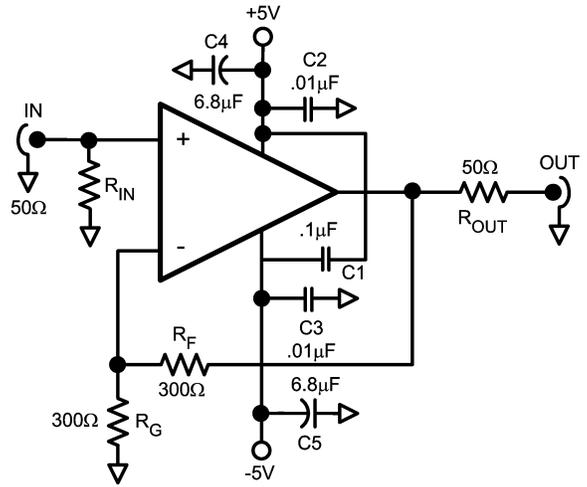
FIGURE 5. Typical Application with Suggested Supply Bypassing
