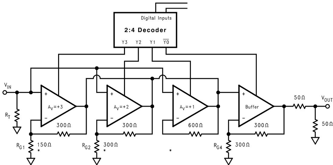
\*NOTE: Selectable gains can be changed by using different  $R_g$  resistors.
