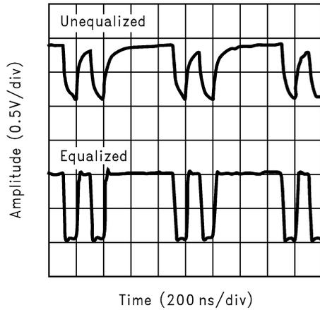
FIGURE 9. Digital Signal without and with Equalization
