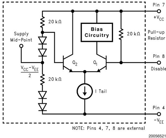
FIGURE 4. Enable/Disable Operation
