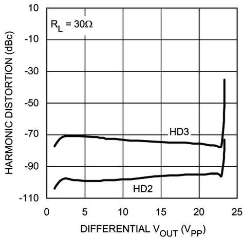
Harmonic Distortion @  $I_{CC} = 21\text{ mA}$ , 1 MHz
