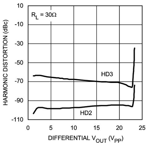
Harmonic Distortion @  $I_{CC} = 11.4\text{ mA}$ , 1 MHz
