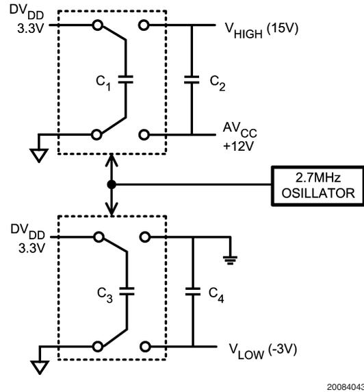
FIGURE 3. Charge Pump Functional Schematic
