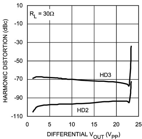
Harmonic Distortion @  $I_{CC} = 16\text{ mA}$ , 1 MHz
