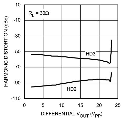
Harmonic Distortion @  $I_{CC} = 11.4\text{ mA}$ , 200 kHz
