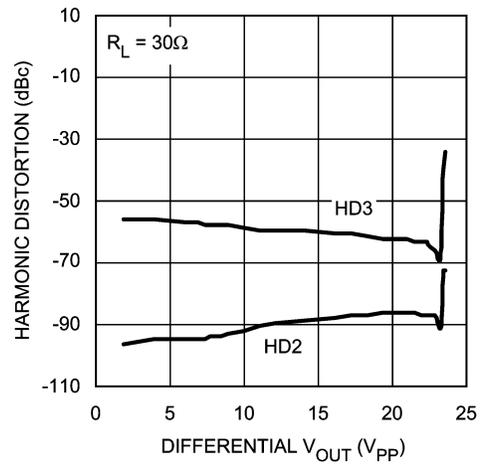
Harmonic Distortion @  $I_{CC} = 16\text{ mA}$ , 200 kHz
