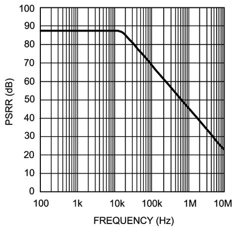
PSRR- vs. Frequency  $V_S = 5V$  and 12V
