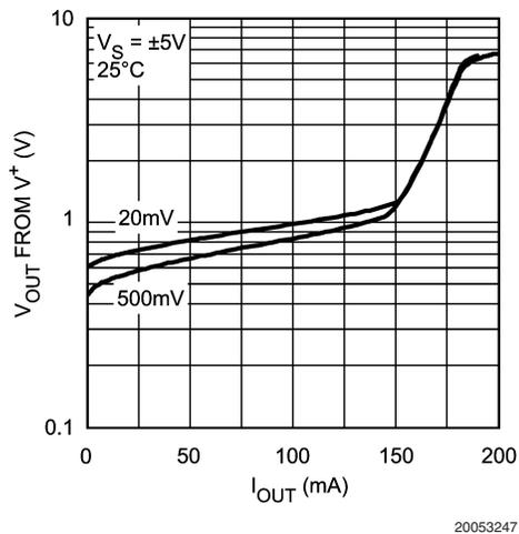
FIGURE 4.  $V_{OUT}$  vs.  $I_{SOURCE}$  (for Various Overdrive)
