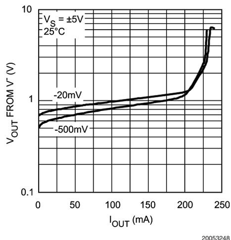
FIGURE 5.  $V_{OUT}$  vs.  $I_{SINK}$  (for Various Overdrive)
