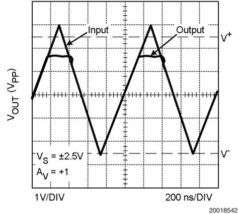
**FIGURE 1. Input and Output Shown with CMVR Exceeded**
