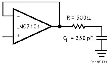
**FIGURE 4. Resistive Isolation of a 330 pF Capacitive Load**
