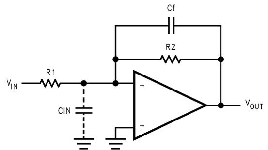
**FIGURE 5. Cancelling the Effect of Input Capacitance**
