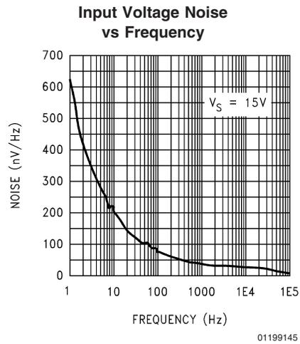
**Typical Performance Characteristics**  $V_S = +15V$ , Single Supply,  $T_A = 25^\circ C$  unless specified (Continued)
