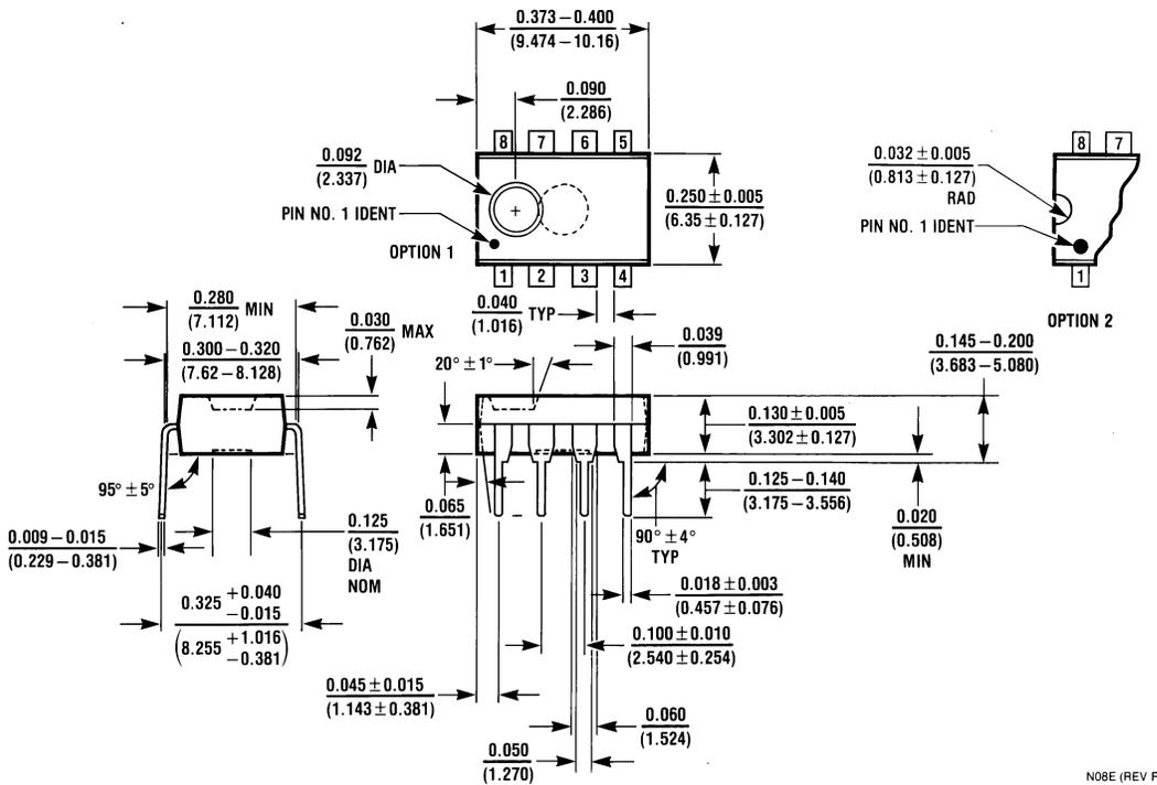
**8-Pin Molded Dual-In-Line Package**
