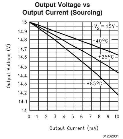
**Typical Performance Characteristics**  $V^+ = 5V$ , Single Supply,  $T_A = 25^\circ C$  unless otherwise specified (Continued)
