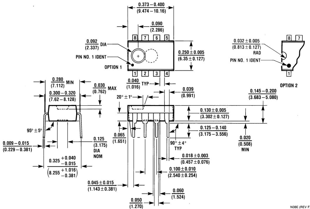
**8-Pin Molded Dual-In-Line Package**
