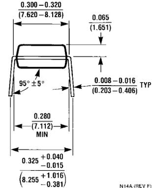
**14-Pin Molded Dual-In-Line Package**
