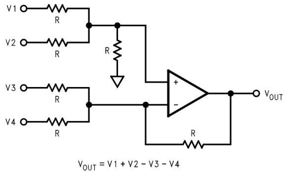
$$V_{OUT} = V_1 + V_2 - V_3 - V_4$$
