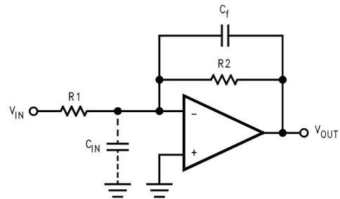
**FIGURE 4. Cancelling the Effect of Input Capacitance**
