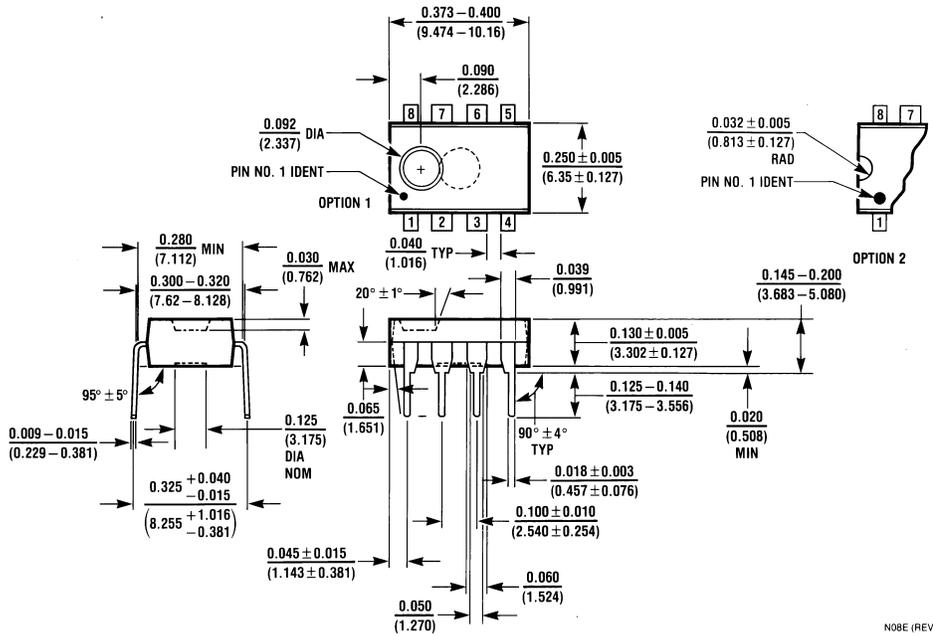
**8-Lead (0.300" Wide) Molded Dual-In-Line Package**
