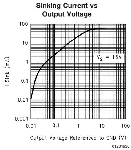
**Typical Performance Characteristics**  $V_S = +15V$ , Single Supply,  $T_A = 25^\circ C$  unless otherwise specified (Continued)
