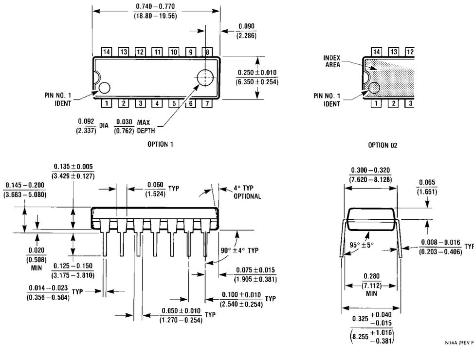
**14-Lead Molded Dual-In-Line Package**
