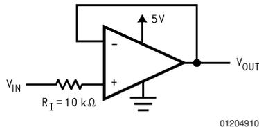
**FIGURE 3. R<sub>I</sub> Input Current Protection for Voltages Exceeding the Supply Voltages**
