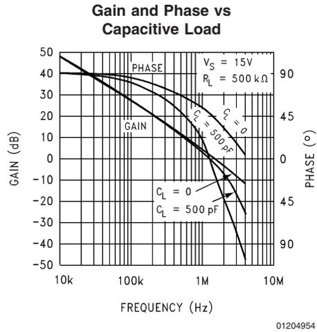
**Typical Performance Characteristics**  $V_S = +15V$ , Single Supply,  $T_A = 25^\circ C$  unless otherwise specified (Continued)
